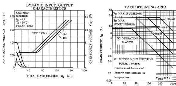
DRAIN-SOURCE VOLTAGE VDS (V)
