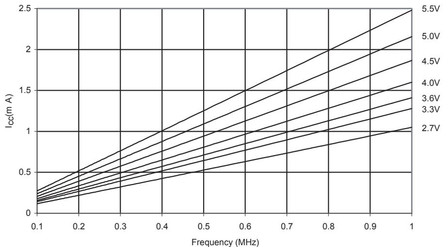
**Figure 164.** Active Supply Current vs. Frequency (1 MHz - 20 MHz)
