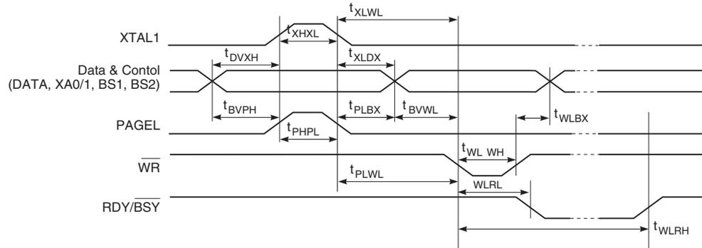
**Figure 145.** Parallel Programming Timing, Loading Sequence with Timing Requirements<sup>(1)</sup>
