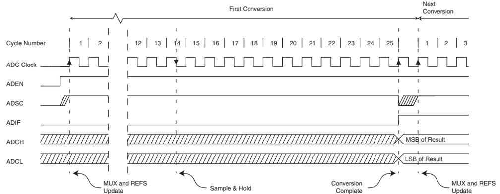
**Figure 112. ADC Timing Diagram, Single Conversion**
