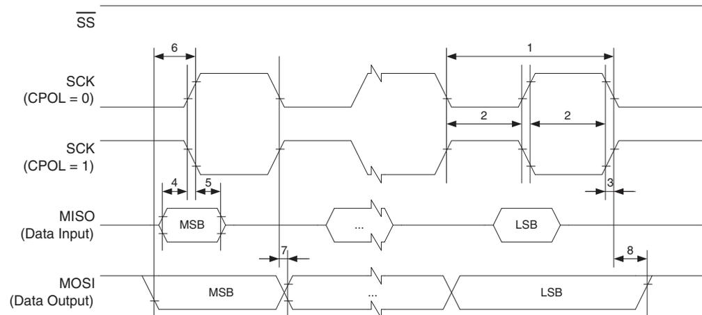
**Figure 158. SPI Interface Timing Requirements (Slave Mode)**
