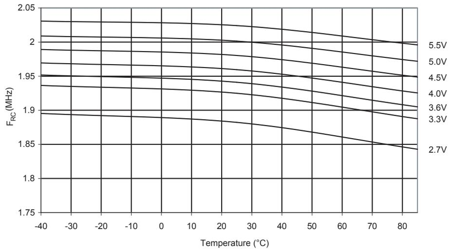
**Figure 206.** Calibrated 2 MHz RC Oscillator Frequency vs.  $V_{CC}$
