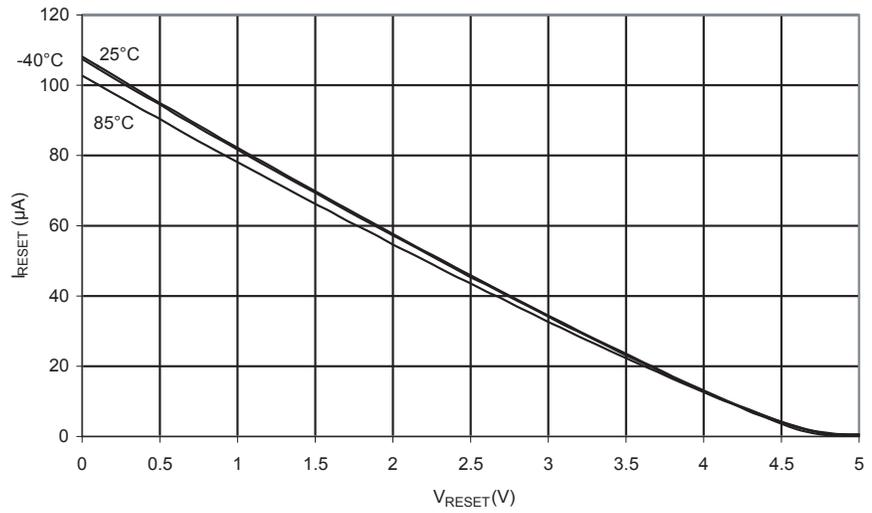
**Figure 185.** Reset Pull-up Resistor Current vs. Reset Pin Voltage ( $V_{CC} = 2.7V$ )
