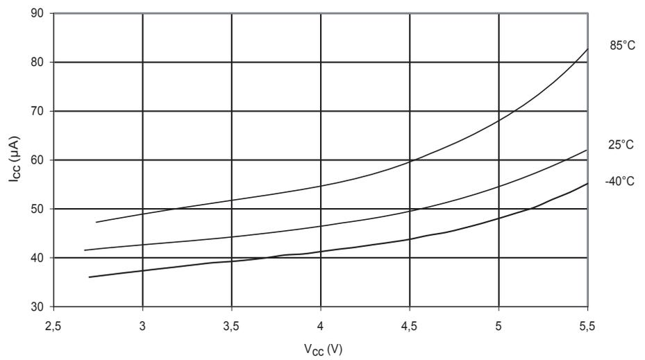
**Figure 218.** Programming Current vs.  $V_{CC}$
