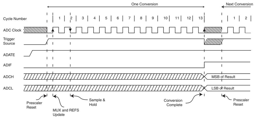
**Figure 114. ADC Timing Diagram, Free Running Conversion**
