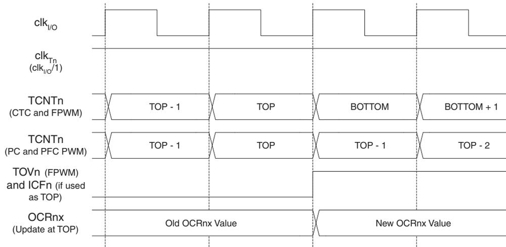
**Figure 58** shows the same timing data, but with the prescaler enabled.
