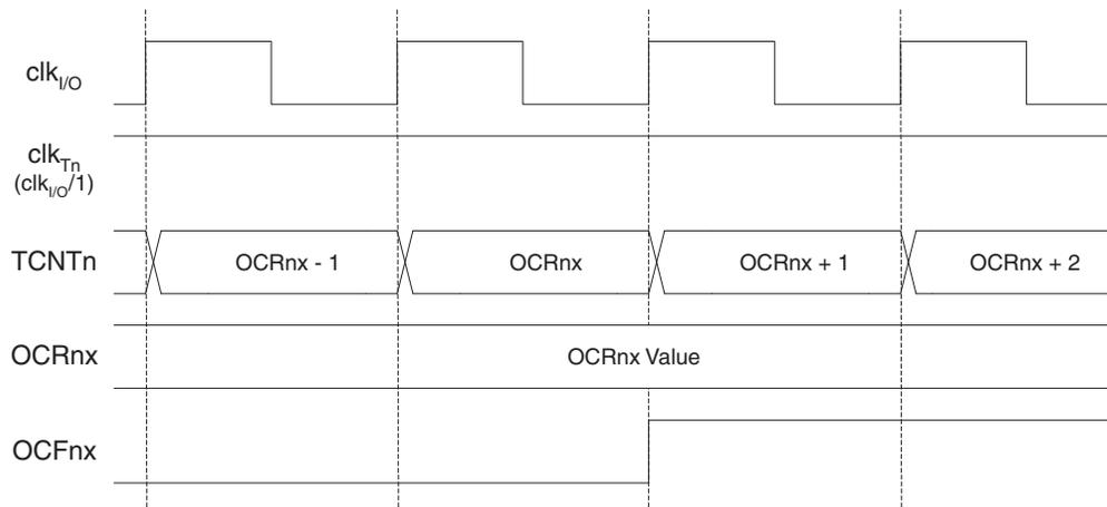
Figure 56 shows the same timing data, but with the prescaler enabled.
