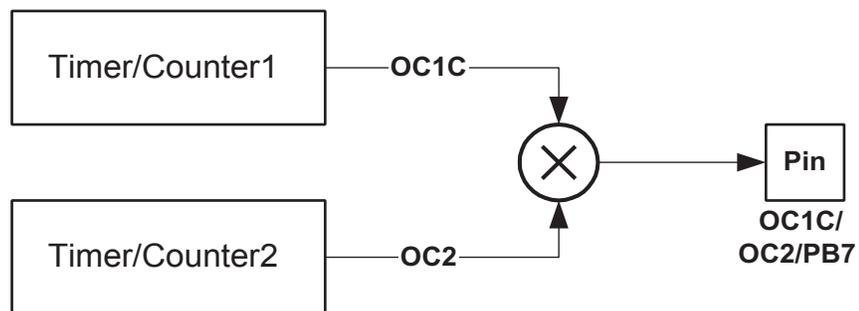
When the modulator is enabled, the two Output Compare channels are modulated together as shown in the block diagram ([Figure 72](#)).
