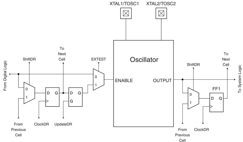
Table 102 summarizes the scan registers for the external clock pin XTAL1, oscillators with XTAL1/XTAL2 connections as well as 32 kHz Timer Oscillator.
