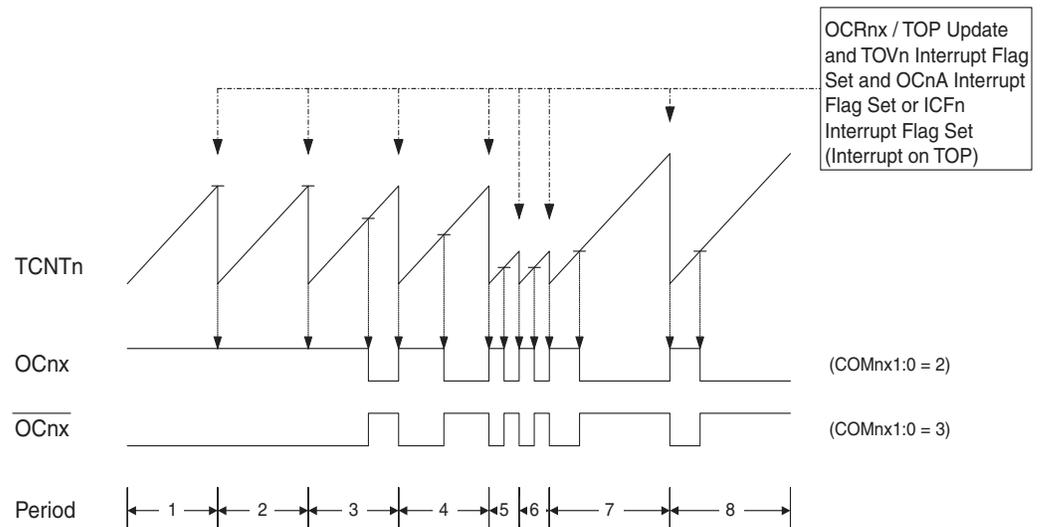
The Timer/Counter Overflow Flag (TOVn) is set each time the counter reaches TOP. In addition the OCnA or ICFn flag is set at the same timer clock cycle as TOVn is set when either OCRnA or ICRn is used for defining the TOP value. If one of the interrupts are enabled, the interrupt handler routine can be used for updating the TOP and compare values.
