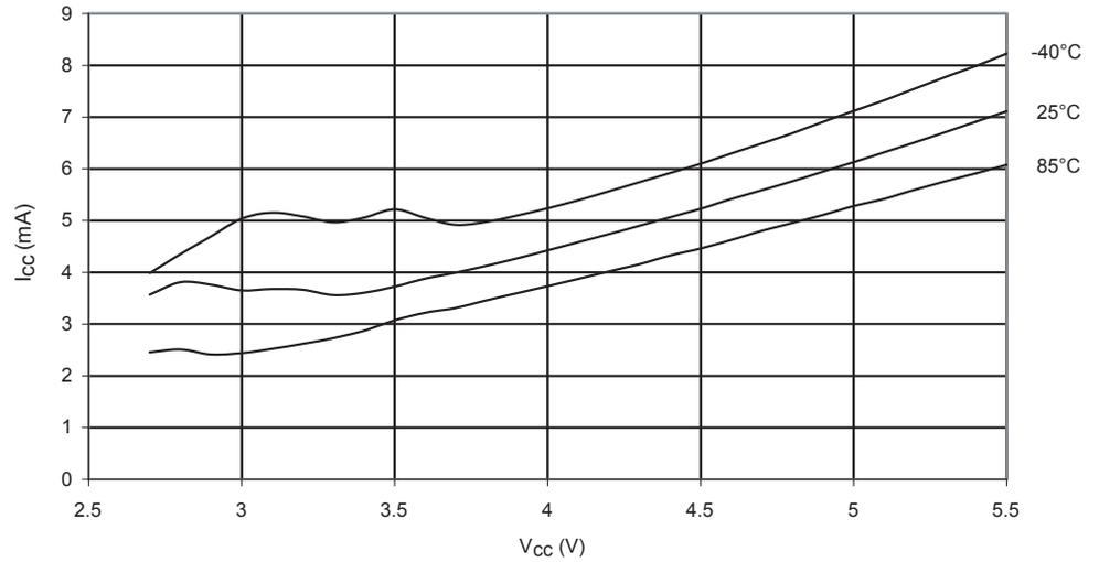
**Current Consumption in Reset and Reset Pulse width**
