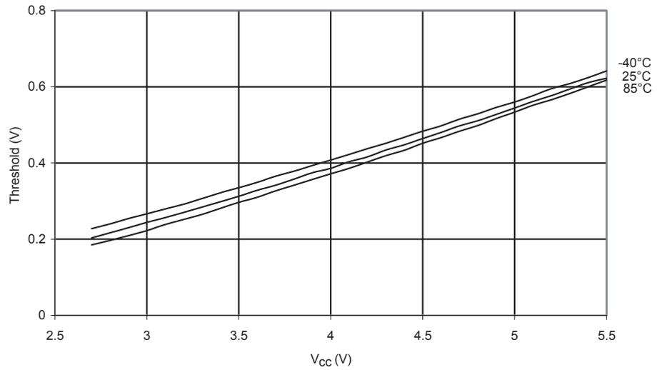
**Figure 195.** Reset Input Threshold Voltage vs.  $V_{CC}$  ( $V_{IH}$ , Reset Pin Read as '1')
