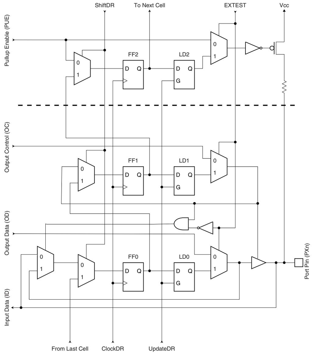
**Figure 128.** General Port Pin Schematic Diagram
