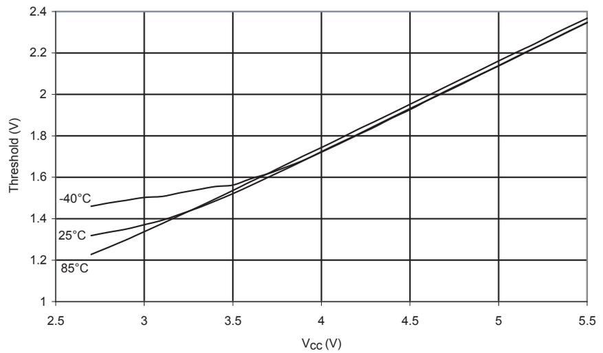
**Figure 196.** Reset Input Threshold Voltage vs.  $V_{CC}$  (VIL, Reset Pin Read as '0')
