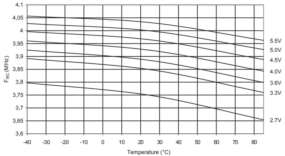
**Figure 209.** Calibrated 4 MHz RC Oscillator Frequency vs. V<sub>CC</sub>
