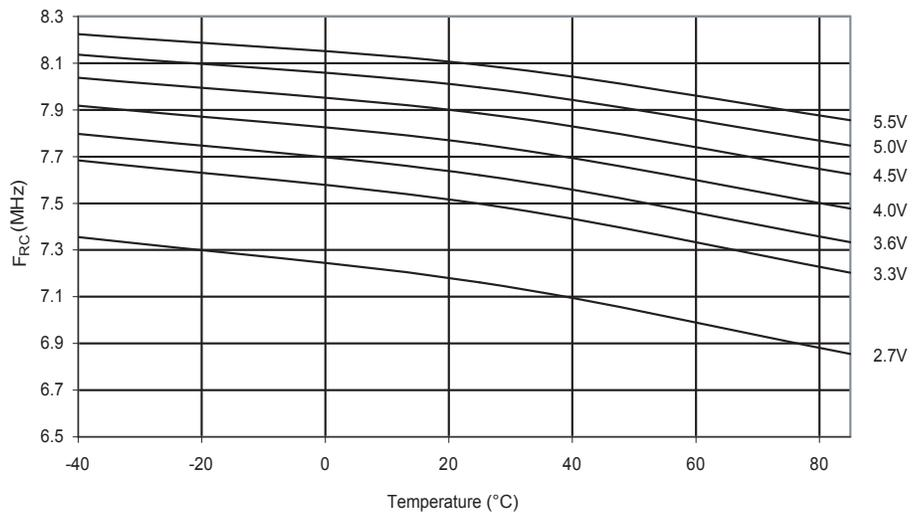
**Figure 212.** Calibrated 8 MHz RC Oscillator Frequency vs.  $V_{CC}$
