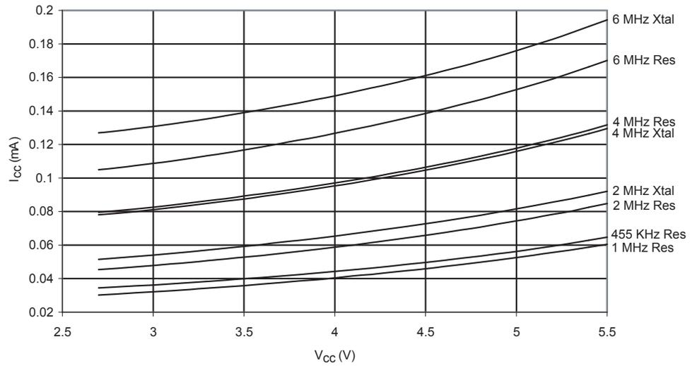
**Figure 181.** Standby Supply Current vs.  $V_{CC}$  (CKOPT Programmed)
