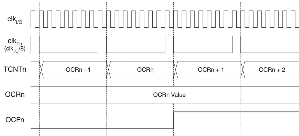
Figure 44 shows the setting of OCF0 and the clearing of TCNT0 in CTC mode.
