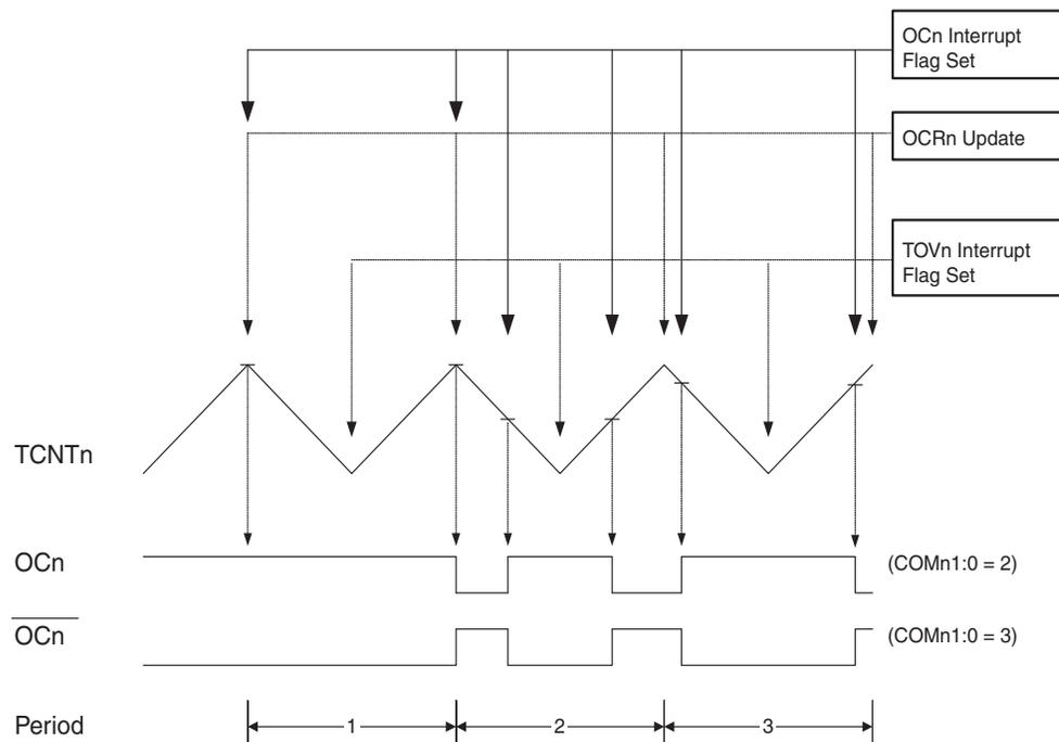
The Timer/Counter Overflow Flag (TOV0) is set each time the counter reaches BOTTOM. The interrupt flag can be used to generate an interrupt each time the counter reaches the BOTTOM value.
