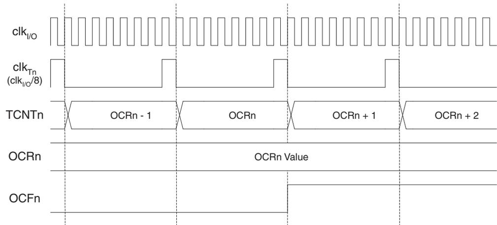
Figure 71 shows the setting of OCF2 and the clearing of TCNT2 in CTC mode.
