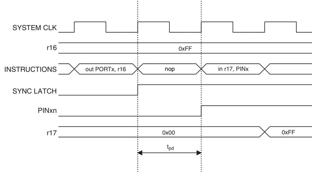
The following code example show how to set Port B pins 0 and 1 high, 2 and 3 low, and define the port pins from 4 to 7 as input with pull-ups assigned to port pins 6 and 7. The resulting pin values are read back again, but as previously discussed, a *nop* instruction is included to be able to read back the value recently assigned to some of the pins.
