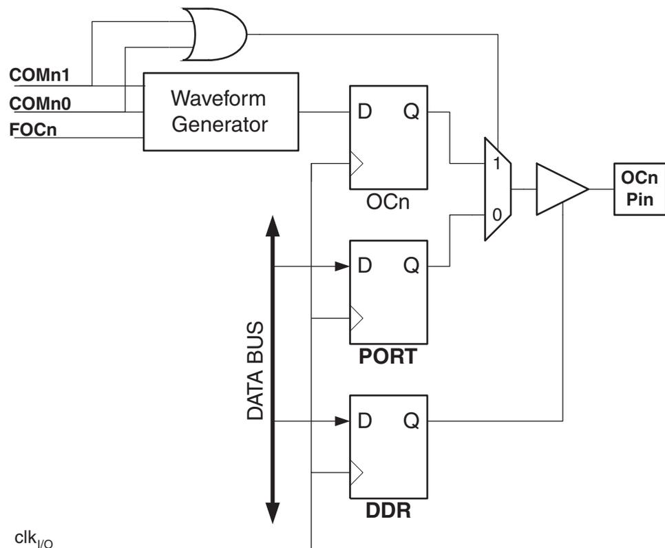
The general I/O port function is overridden by the Output Compare (OC0) from the Waveform Generator if either of the COM01:0 bits are set. However, the OC0 pin direction (input or output) is still controlled by the Data Direction Register (DDR) for the port pin. The Data Direction Register bit for the OC0 pin (DDR\_OC0) must be set as output before the OC0 value is visible on the pin. The port override function is independent of the Waveform Generation mode.
