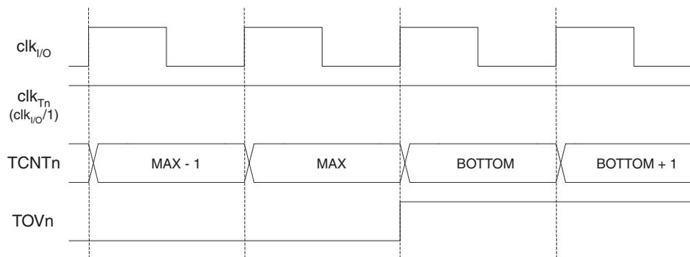
[Figure 42](#) shows the same timing data, but with the prescaler enabled.
