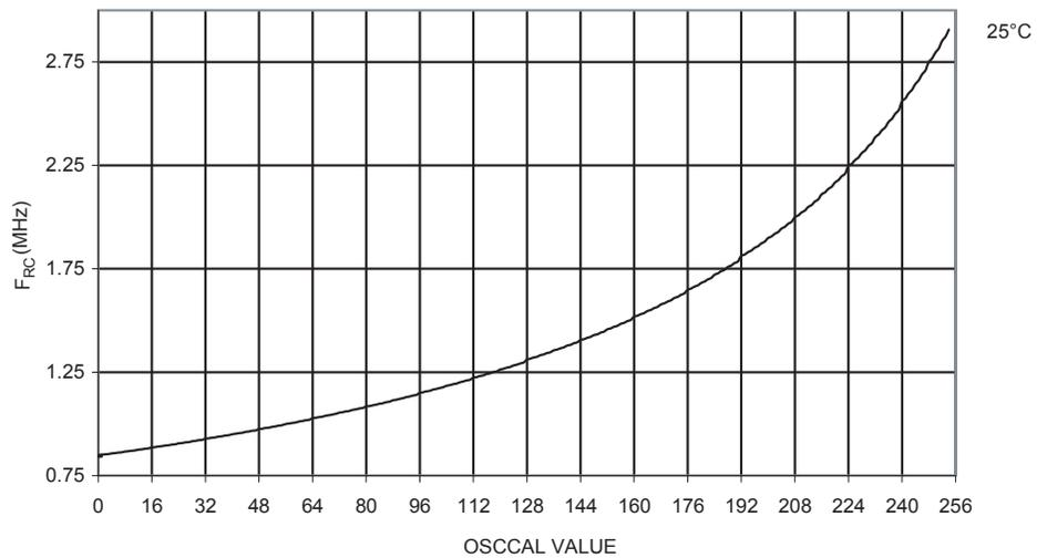
**Figure 208.** Calibrated 4 MHz RC Oscillator Frequency vs. Temperature
