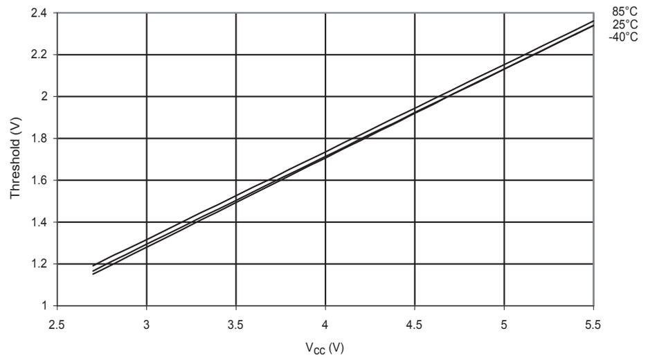
**Figure 197.** Reset Input Pin Hysteresis vs.  $V_{CC}$
