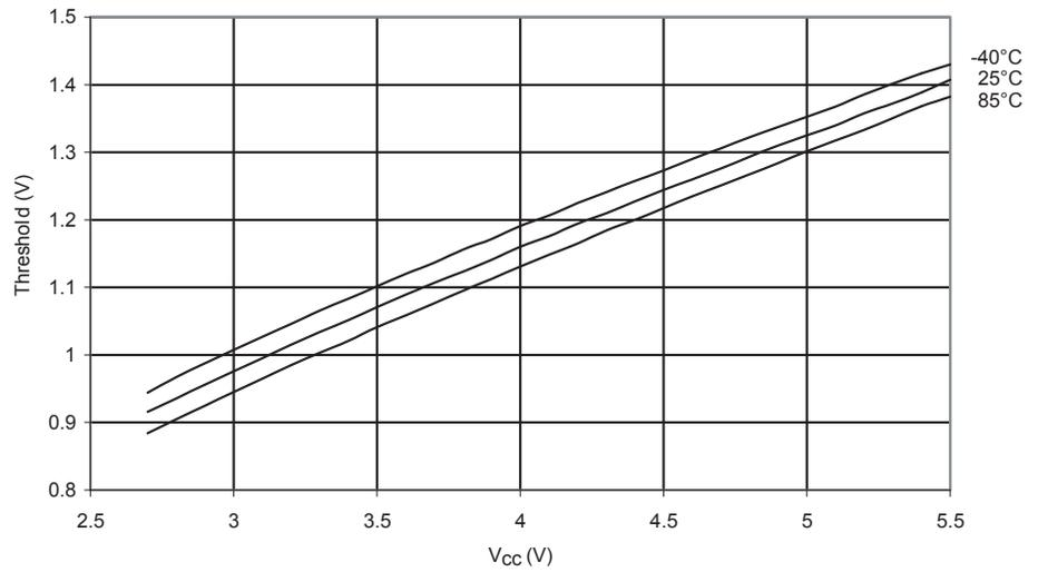
**Figure 194.** I/O Pin Input Hysteresis vs.  $V_{CC}$
