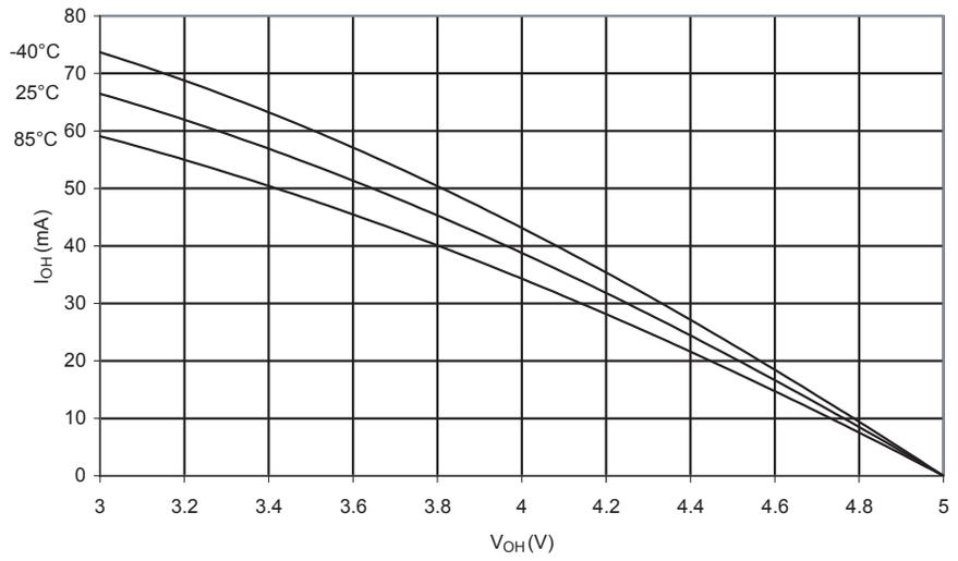
**Figure 189.** I/O Pin Source Current vs. Output Voltage ( $V_{CC} = 2.7V$ )
