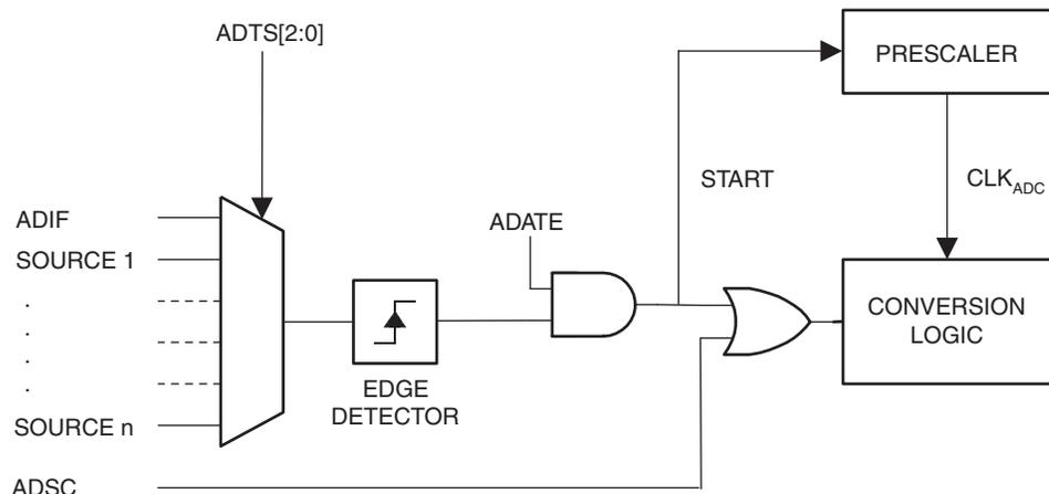
Using the ADC Interrupt Flag as a trigger source makes the ADC start a new conversion as soon as the ongoing conversion has finished. The ADC then operates in Free Running mode, constantly sampling and updating the ADC Data Register. The first conversion must be started by writing a logical one to the ADSC bit in ADCSRA. In this mode the ADC will perform successive conversions independently of whether the ADC Interrupt Flag, ADIF, is cleared or not.
