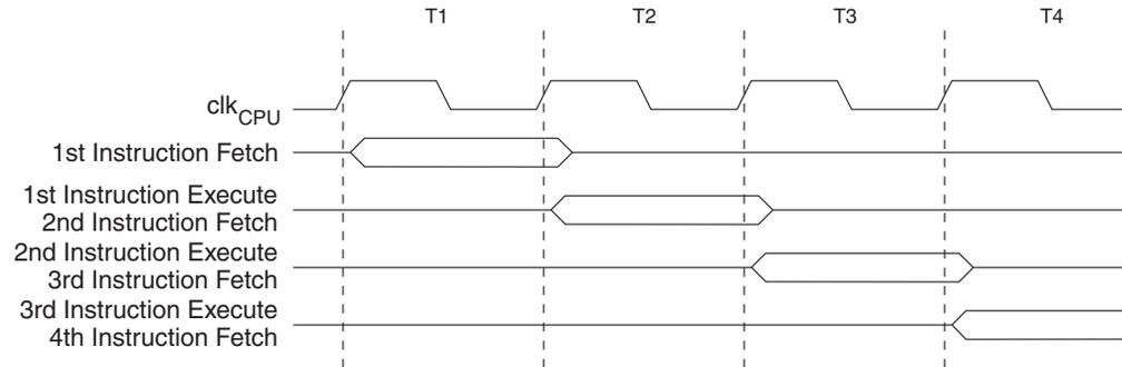
Figure 7 shows the internal timing concept for the Register File. In a single clock cycle an ALU operation using two register operands is executed, and the result is stored back to the destination register.
