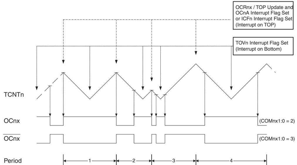
The Timer/Counter Overflow Flag (TOVn) is set each time the counter reaches BOTTOM. When either OCRnA or ICFn is used for defining the TOP value, the OCnA or ICFn flag is set accordingly at the same timer clock cycle as the OCRnx Registers are updated with the double buffer value (at TOP). The interrupt flags can be used to generate an interrupt each time the counter reaches the TOP or BOTTOM value.
