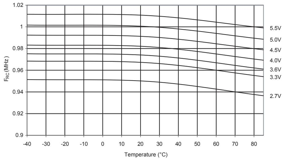
**Figure 203.** Calibrated 1 MHz RC Oscillator Frequency vs. V<sub>CC</sub>
