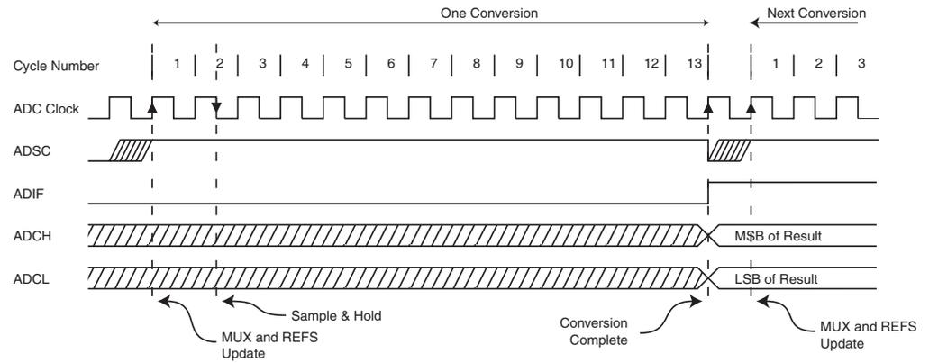
**Figure 113. ADC Timing Diagram, Auto Triggered Conversion**
