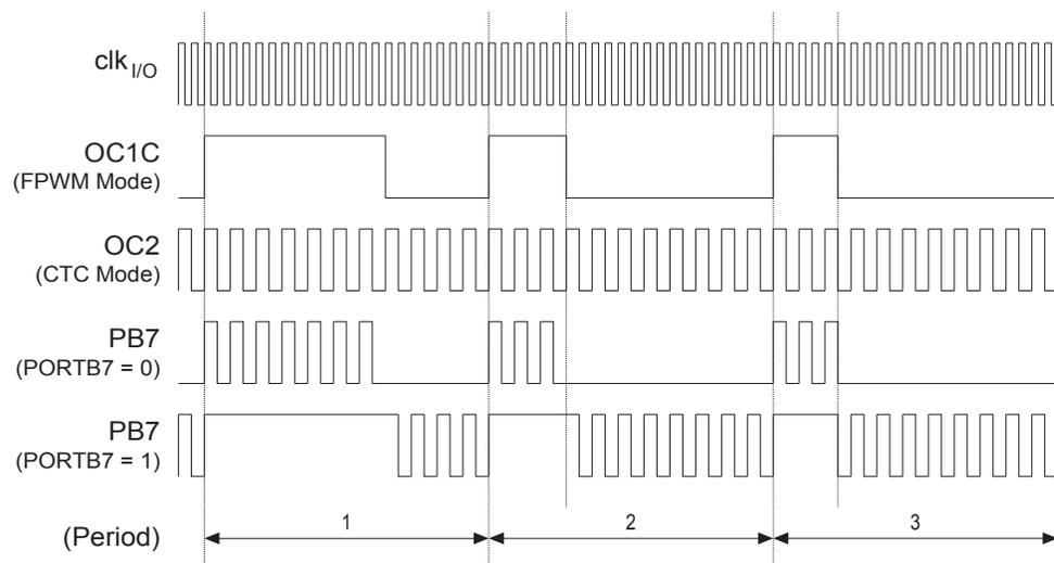
In this example, Timer/Counter2 provides the carrier, while the modulating signal is generated by the Output Compare unit C of the Timer/Counter1.
