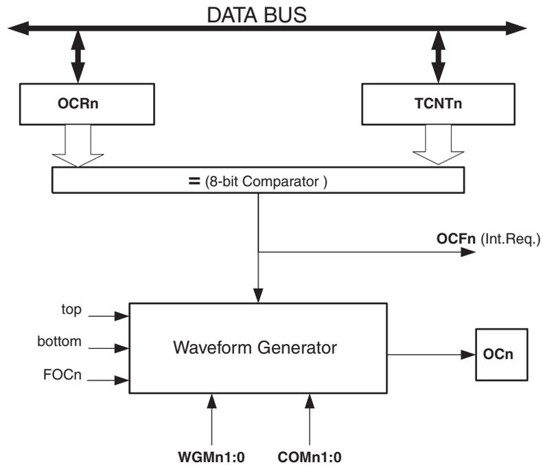
The OCR2 Register is double buffered when using any of the Pulse Width Modulation (PWM) modes. For the normal and Clear Timer on Compare (CTC) modes of operation, the double buffering is disabled. The double buffering synchronizes the update of the OCR2 Compare Register to either top or bottom of the counting sequence. The synchronization prevents the occurrence of odd-length, non-symmetrical PWM pulses, thereby making the output glitch-free.
