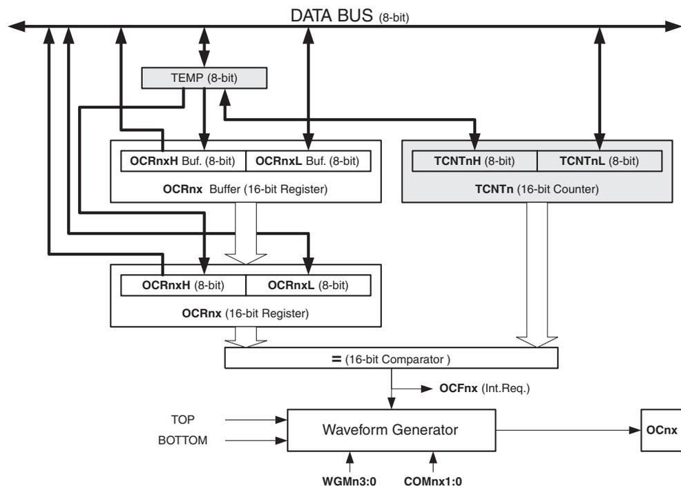
The OCRnx Register is double buffered when using any of the twelve *Pulse Width Modulation* (PWM) modes. For the normal and *Clear Timer on Compare* (CTC) modes of operation, the double buffering is disabled. The double buffering synchronizes the update of the OCRnx Compare Register to either TOP or BOTTOM of the counting sequence. The synchronization prevents the occurrence of odd-length, non-symmetrical PWM pulses, thereby making the output glitch-free.
