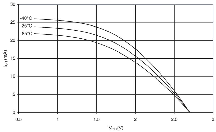
**Figure 190.** I/O Pin Sink Current vs. Output Voltage ( $V_{CC} = 5V$ )
