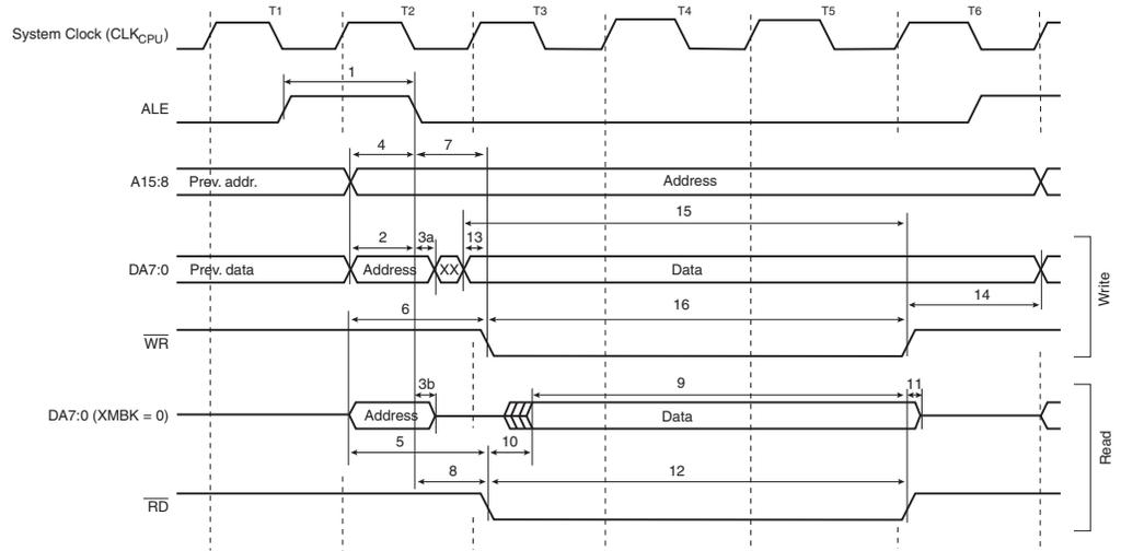
**Figure 162. External Memory Timing (SRWn1 = 1, SRWn0 = 1)<sup>(1)</sup>**
