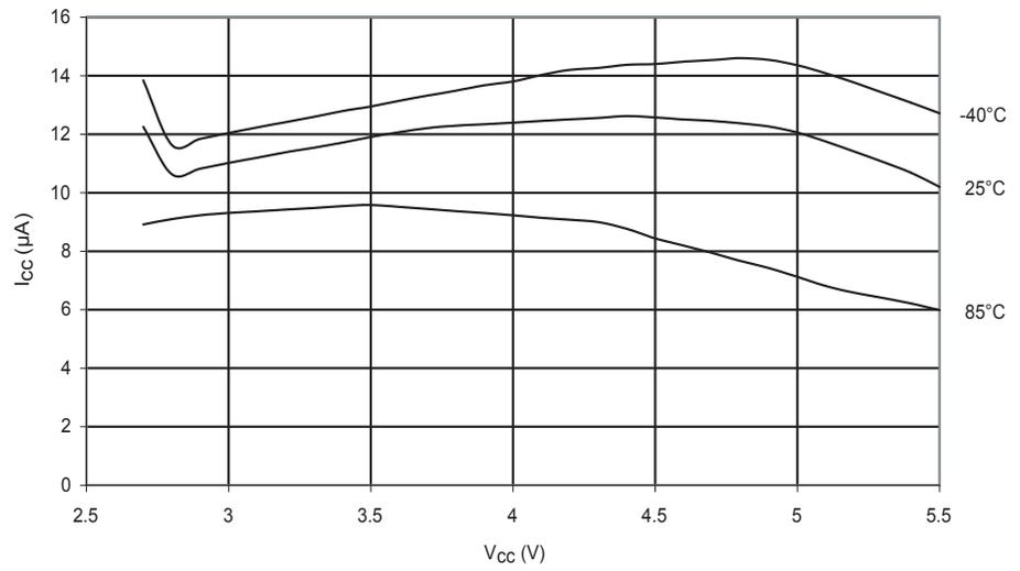
**Figure 215. ADC Current vs.  $V_{CC}$  (ADC CLK = 50 kHz)**
