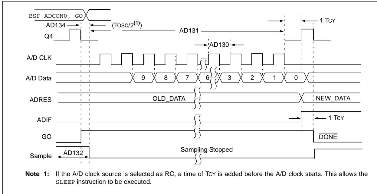
**FIGURE 17-11: PIC16F882/883/884/886/887 A/D CONVERSION TIMING (SLEEP MODE)**
