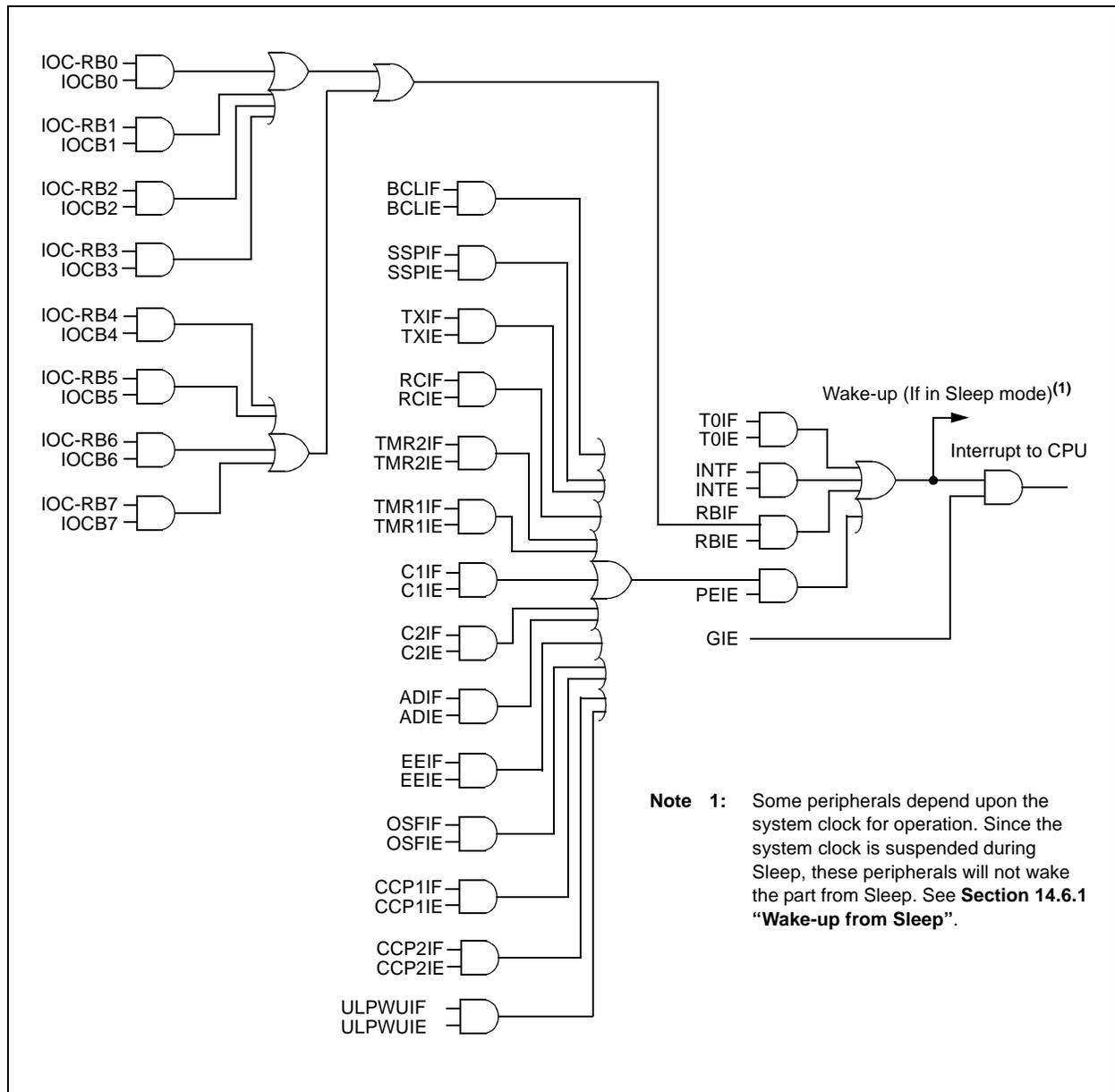
**Note 1:** Some peripherals depend upon the system clock for operation. Since the system clock is suspended during Sleep, these peripherals will not wake the part from Sleep. See **Section 14.6.1 “Wake-up from Sleep”**.
