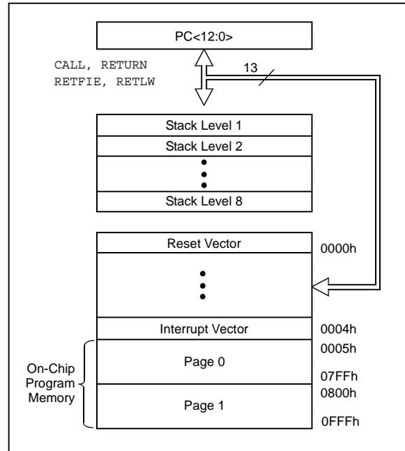
**FIGURE 2-3: PROGRAM MEMORY MAP AND STACK FOR THE PIC16F886/PIC16F887**
