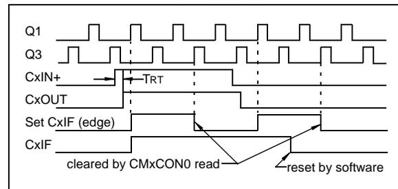
**Note 1:** If a change in the CMxCON0 register (CxOUT) should occur when a read operation is being executed (start of the Q2 cycle), then the CxIF of the PIR2 register interrupt flag may not get set.
