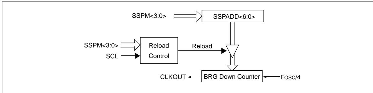
**FIGURE 13-12: BAUD RATE GENERATOR TIMING WITH CLOCK ARBITRATION**
