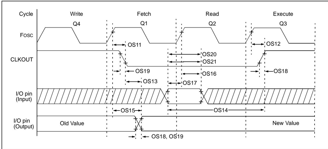
**TABLE 17-3: CLKOUT AND I/O TIMING PARAMETERS**
