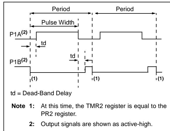
**FIGURE 11-9: EXAMPLE OF HALF-BRIDGE APPLICATIONS**
