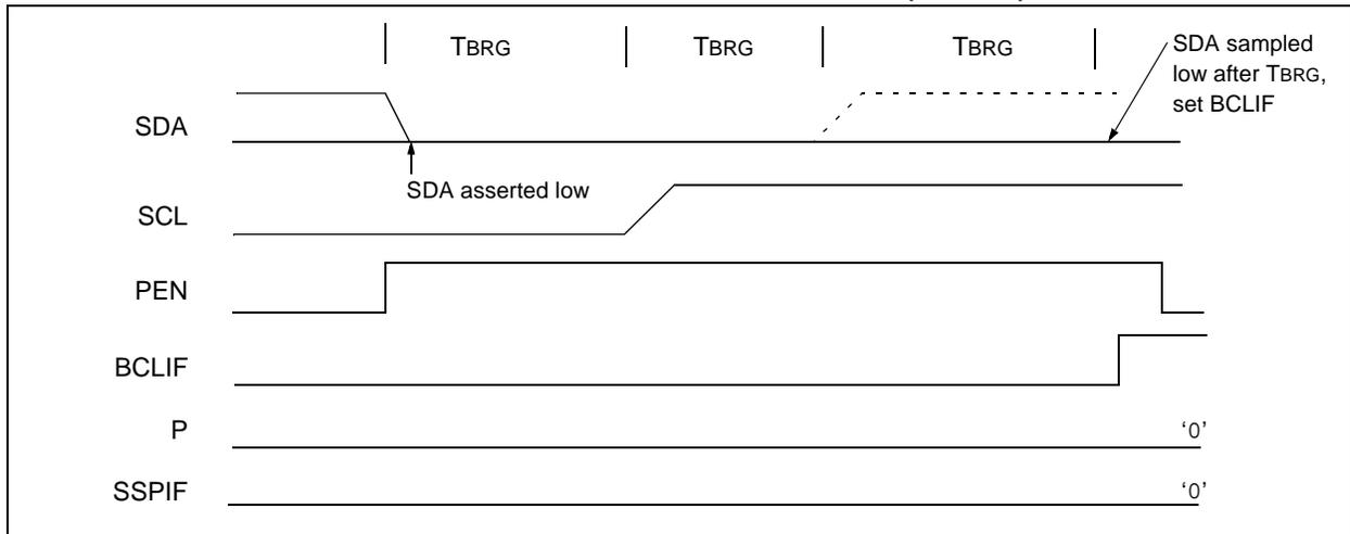
**FIGURE 13-27: BUS COLLISION DURING A STOP CONDITION (CASE 2)**
