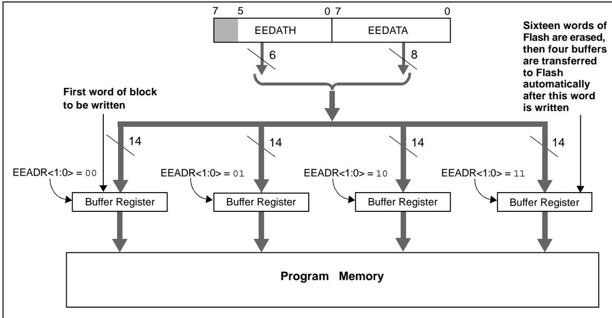
**FIGURE 10-3: BLOCK WRITES TO 8K FLASH PROGRAM MEMORY**
