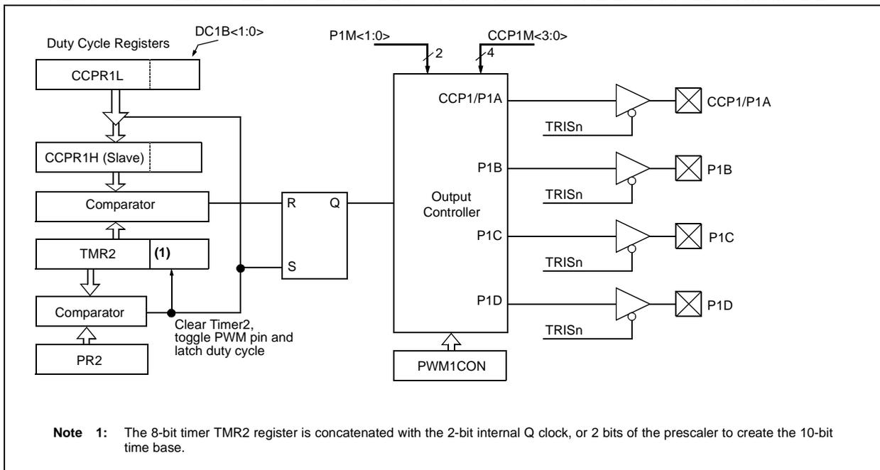
**Note 1:** The TRIS register value for each PWM output must be configured appropriately.
