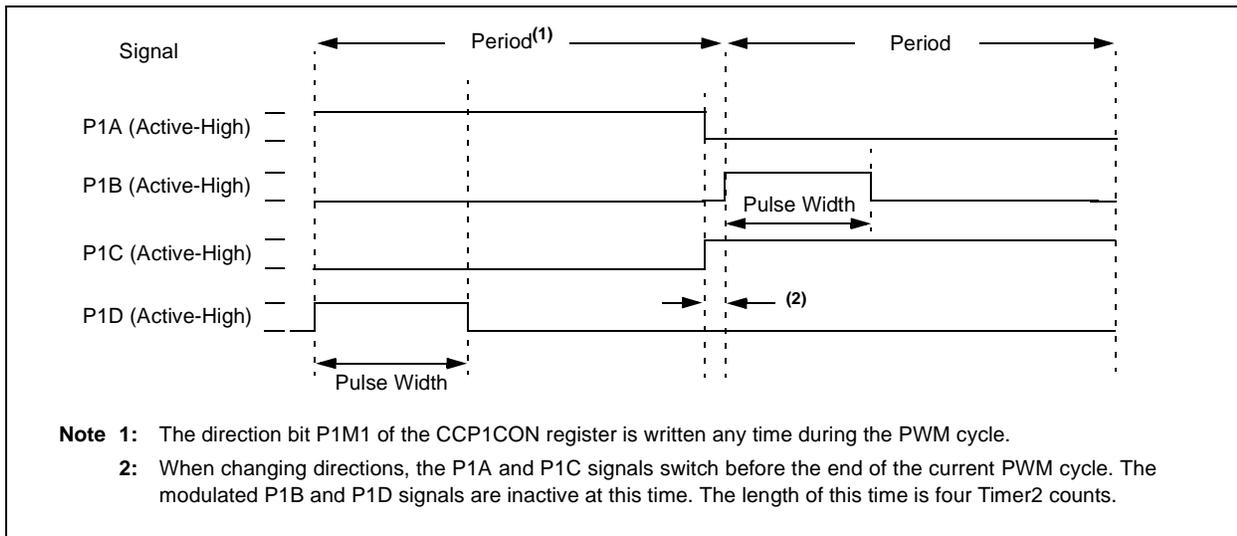
**FIGURE 11-13: EXAMPLE OF PWM DIRECTION CHANGE AT NEAR 100% DUTY CYCLE**
