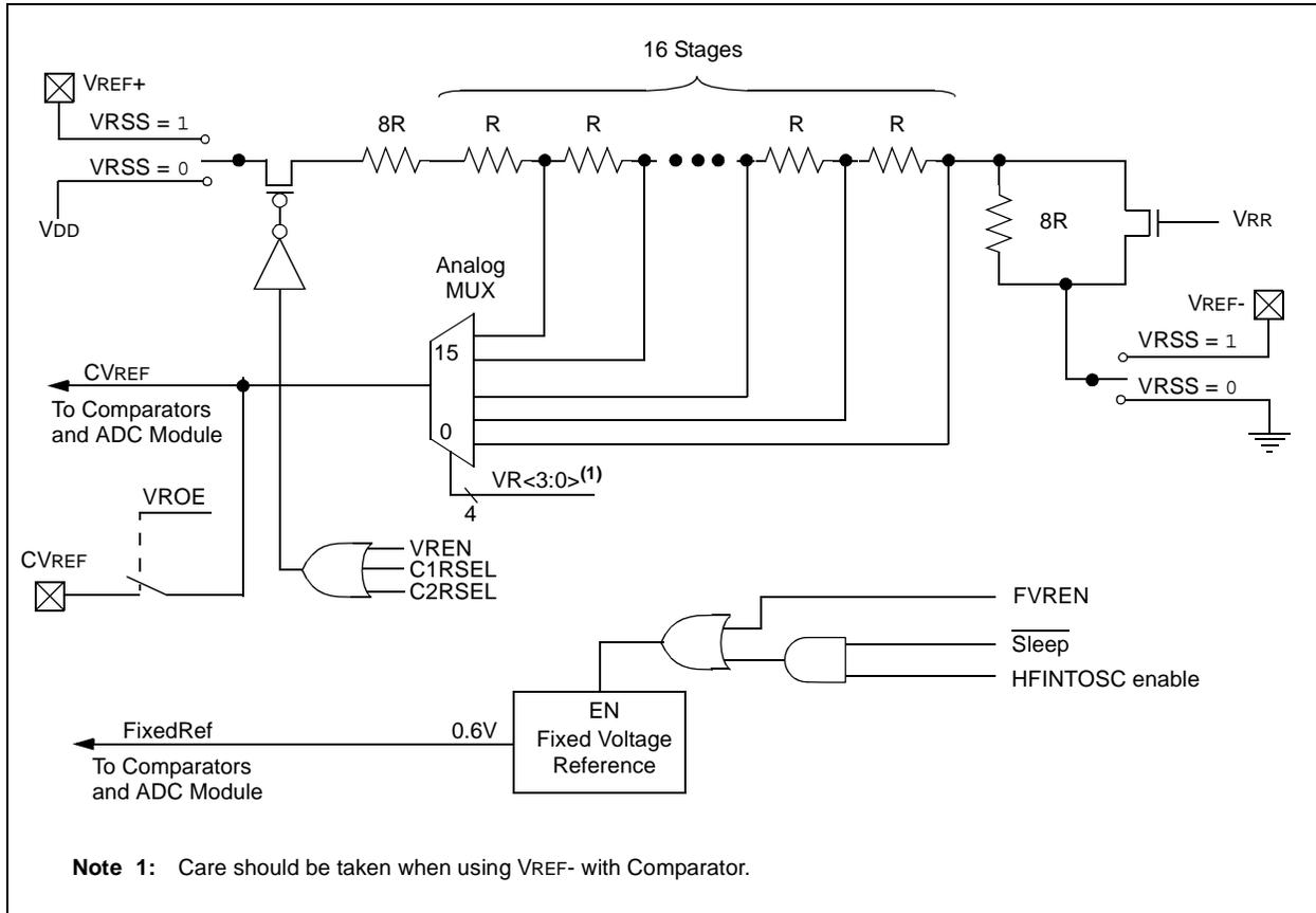
**FIGURE 8-9: COMPARATOR AND ADC VOLTAGE REFERENCE BLOCK DIAGRAM**
