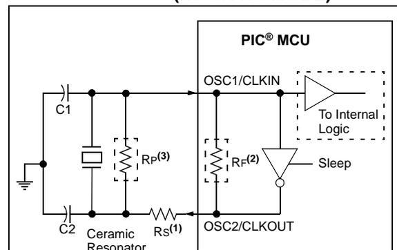
**Note 1:** A series resistor ( $R_S$ ) may be required for ceramic resonators with low drive level.
