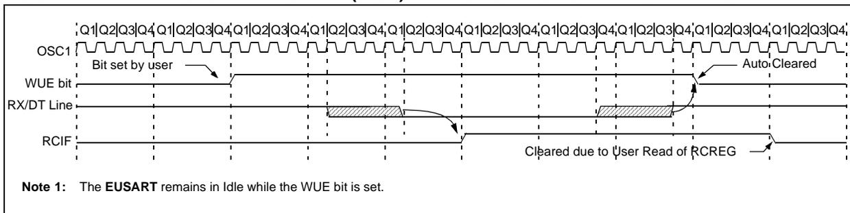
**FIGURE 12-8: AUTO-WAKE-UP BIT (WUE) TIMINGS DURING SLEEP**
