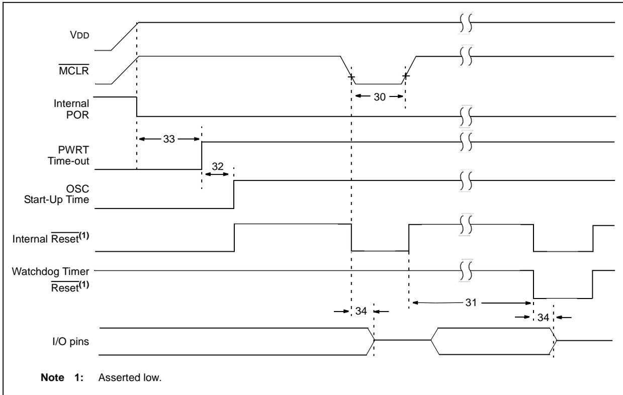
**FIGURE 17-7: BROWN-OUT RESET TIMING AND CHARACTERISTICS**
