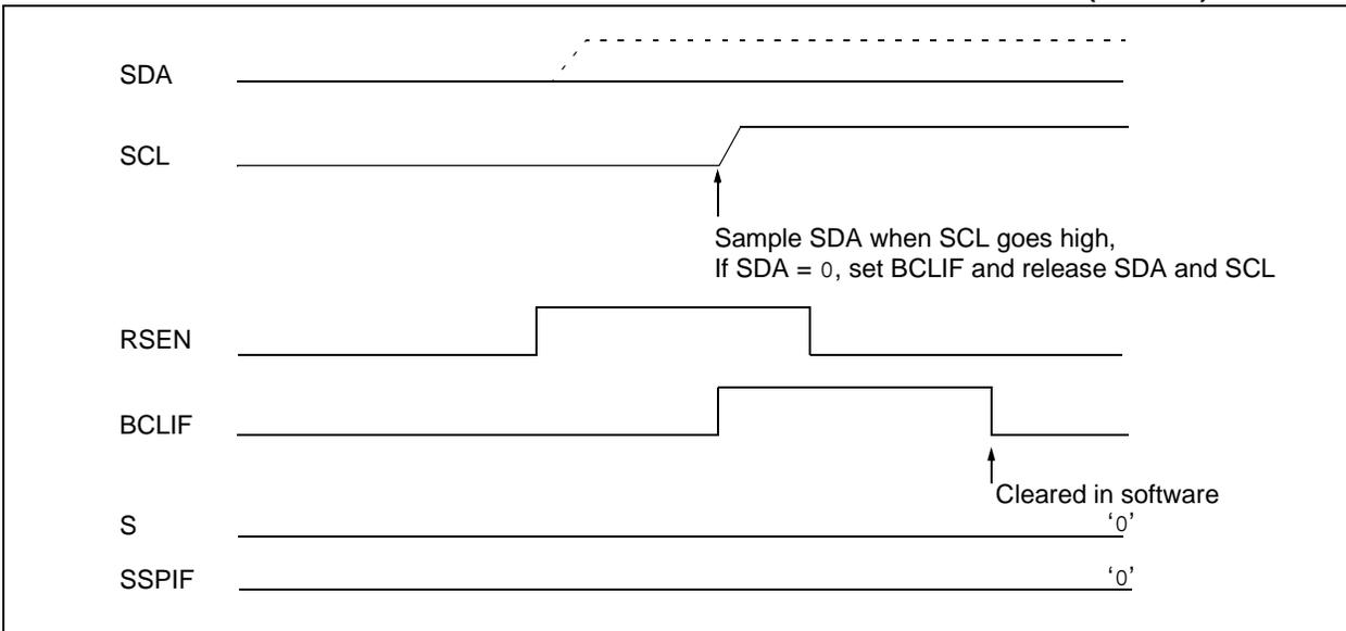
**FIGURE 13-25: BUS COLLISION DURING REPEATED START CONDITION (CASE 2)**
