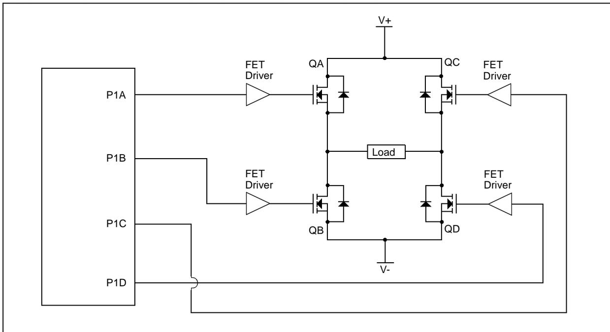
**FIGURE 11-11: EXAMPLE OF FULL-BRIDGE PWM OUTPUT**
