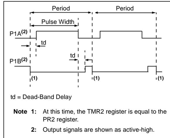
**FIGURE 11-17: EXAMPLE OF HALF-BRIDGE APPLICATIONS**
