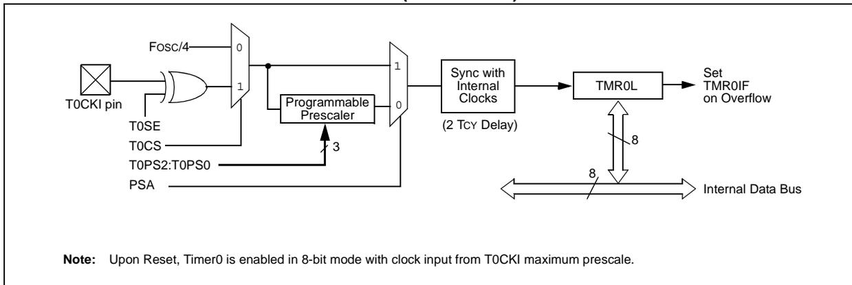
**FIGURE 11-2: TIMER0 BLOCK DIAGRAM (16-BIT MODE)**
