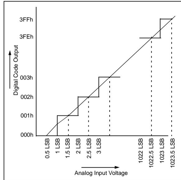
**FIGURE 21-3: ANALOG INPUT MODEL**
