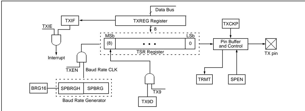
**FIGURE 20-4: ASYNCHRONOUS TRANSMISSION, TXCKP = 0 (TX NOT INVERTED)**
