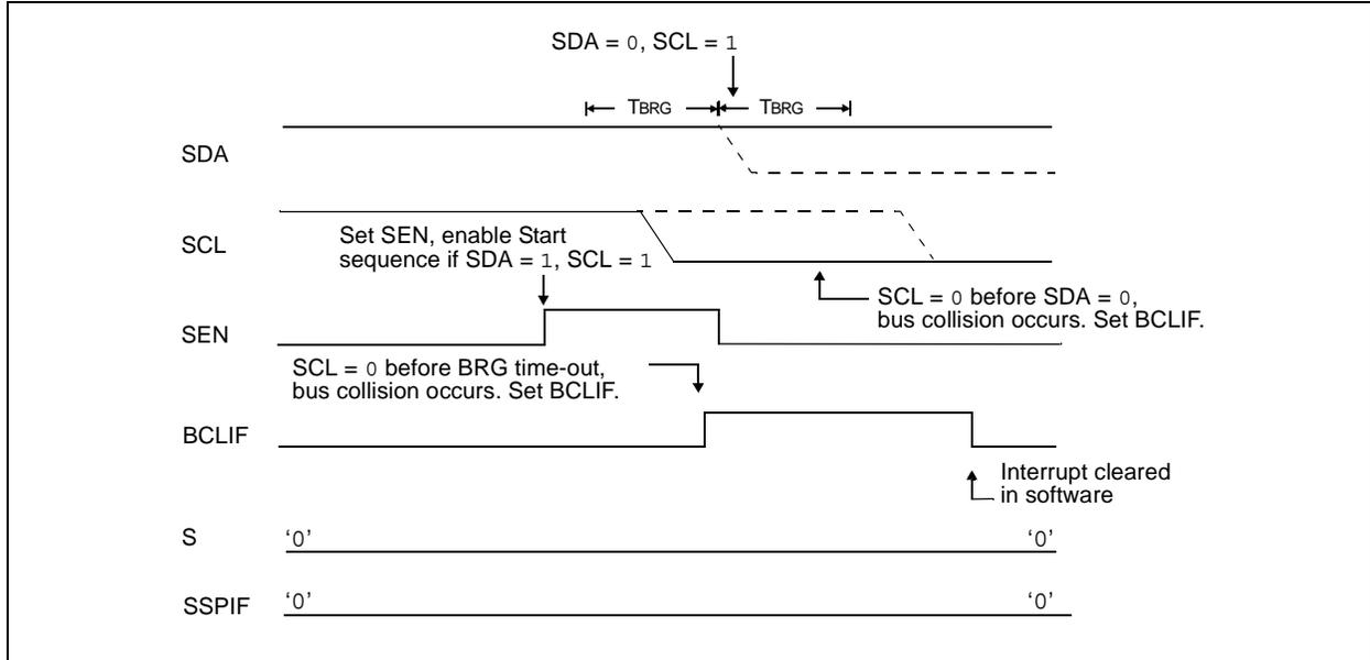
**FIGURE 19-30: BRG RESET DUE TO SDA ARBITRATION DURING START CONDITION**
