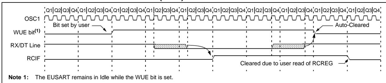
**FIGURE 20-9: AUTO-WAKE-UP BIT (WUE) TIMINGS DURING SLEEP**
