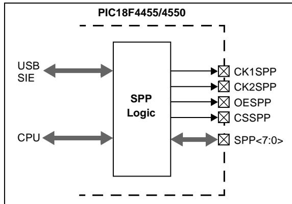
In addition, the SPP can provide time multiplexed addressing information along with the data by using the second strobe output. Thus, the USB endpoint number can be written in conjunction with the data for that endpoint.
