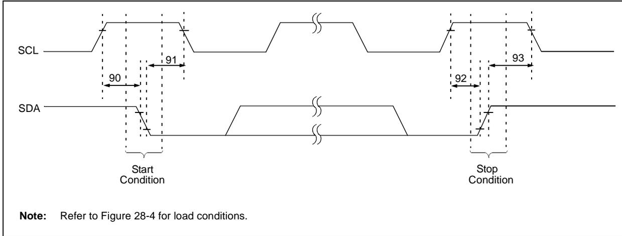
**TABLE 28-21: MASTER SSP I<sup>2</sup>C™ BUS START/STOP BITS REQUIREMENTS**
