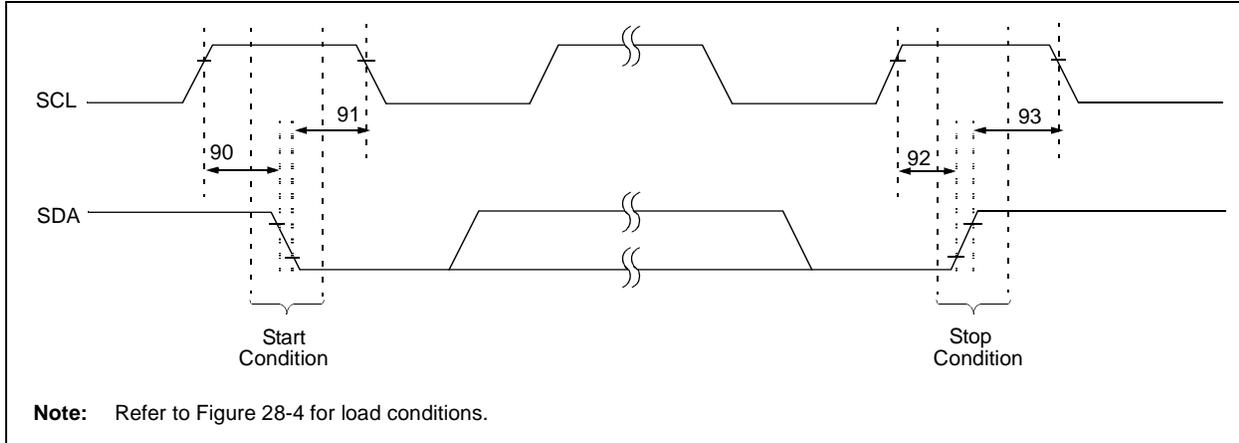
**TABLE 28-19: I<sup>2</sup>C™ BUS START/STOP BITS REQUIREMENTS (SLAVE MODE)**
