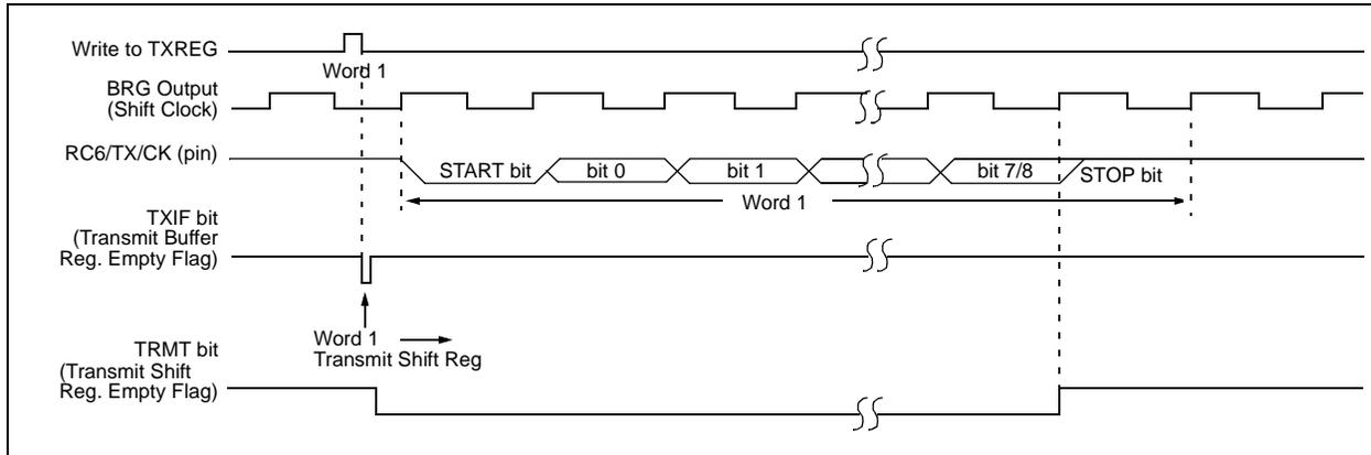
**FIGURE 16-3: ASYNCHRONOUS TRANSMISSION (BACK TO BACK)**
