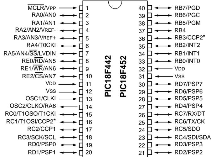
**Note:** Pin compatible with 40-pin PIC16C7X devices.
