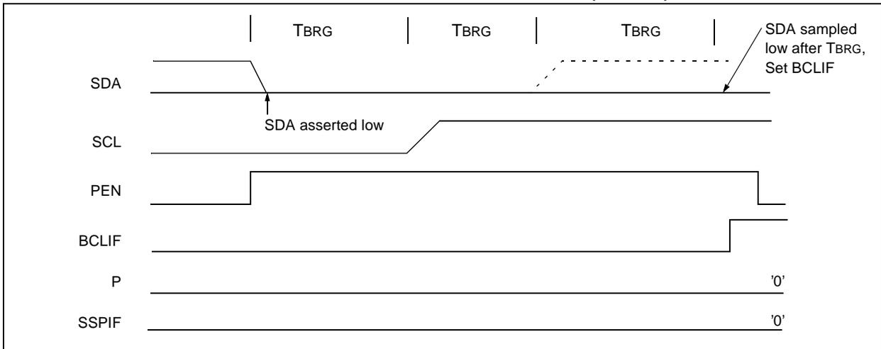
**FIGURE 15-32: BUS COLLISION DURING A STOP CONDITION (CASE 2)**
