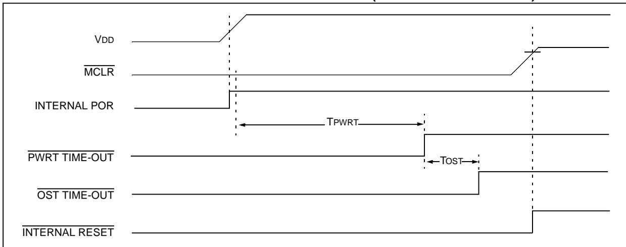
**FIGURE 3-6: SLOW RISE TIME ( $\overline{\text{MCLR}}$  TIED TO  $V_{\text{DD}}$ )**
