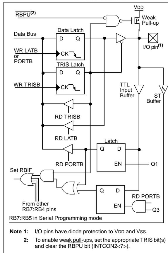
**Note 1:** While in Low Voltage ICSP mode, the RB5 pin can no longer be used as a general purpose I/O pin, and should be held low during normal operation to protect against inadvertent ICSP mode entry.
