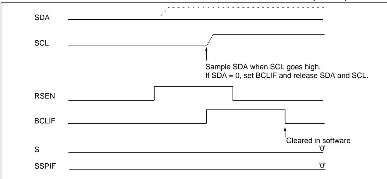
**FIGURE 15-30: BUS COLLISION DURING REPEATED START CONDITION (CASE 2)**
