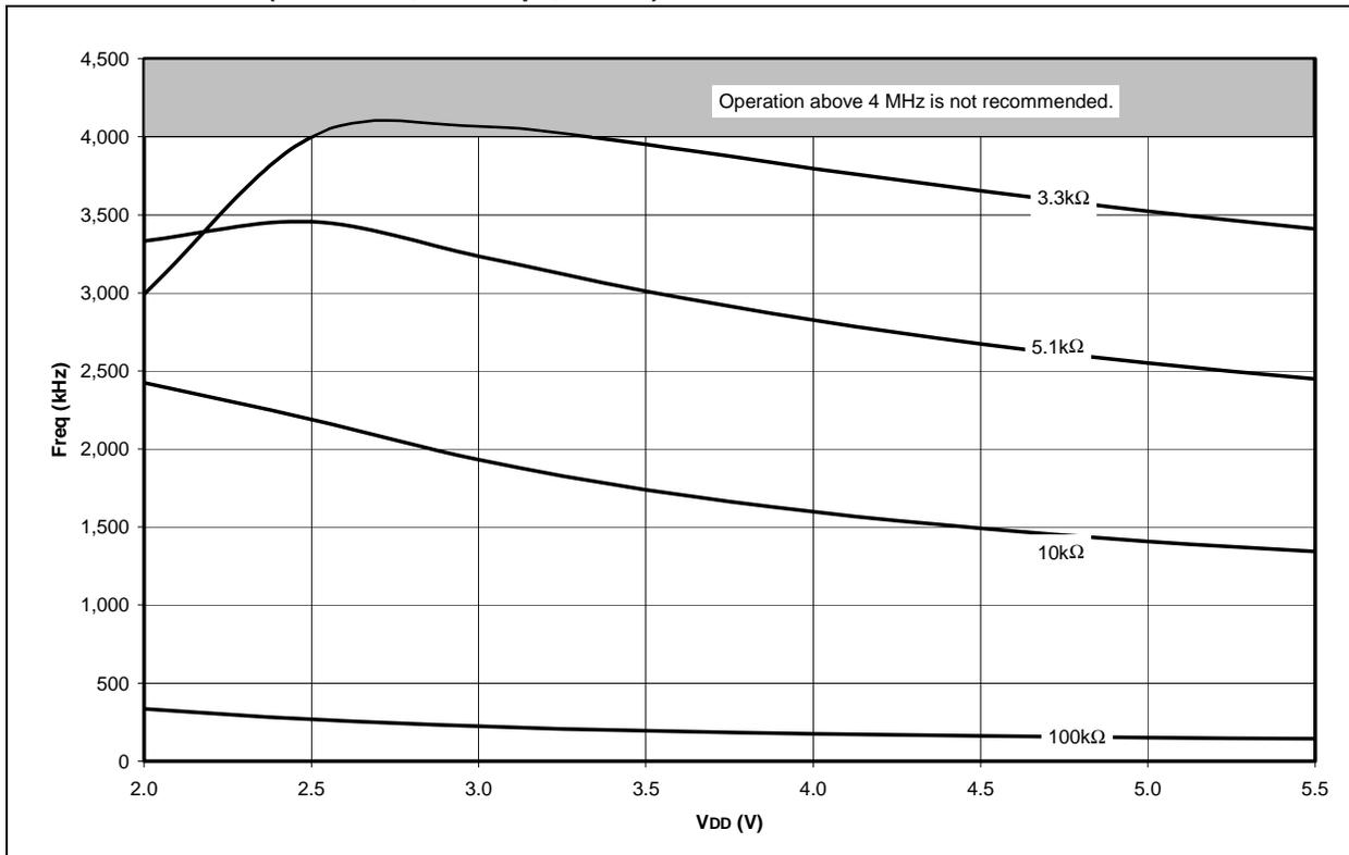
**FIGURE 23-13: AVERAGE  $F_{osc}$  vs.  $V_{DD}$  FOR VARIOUS VALUES OF R
