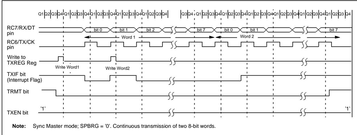
**FIGURE 16-7: SYNCHRONOUS TRANSMISSION (THROUGH TXEN)**
