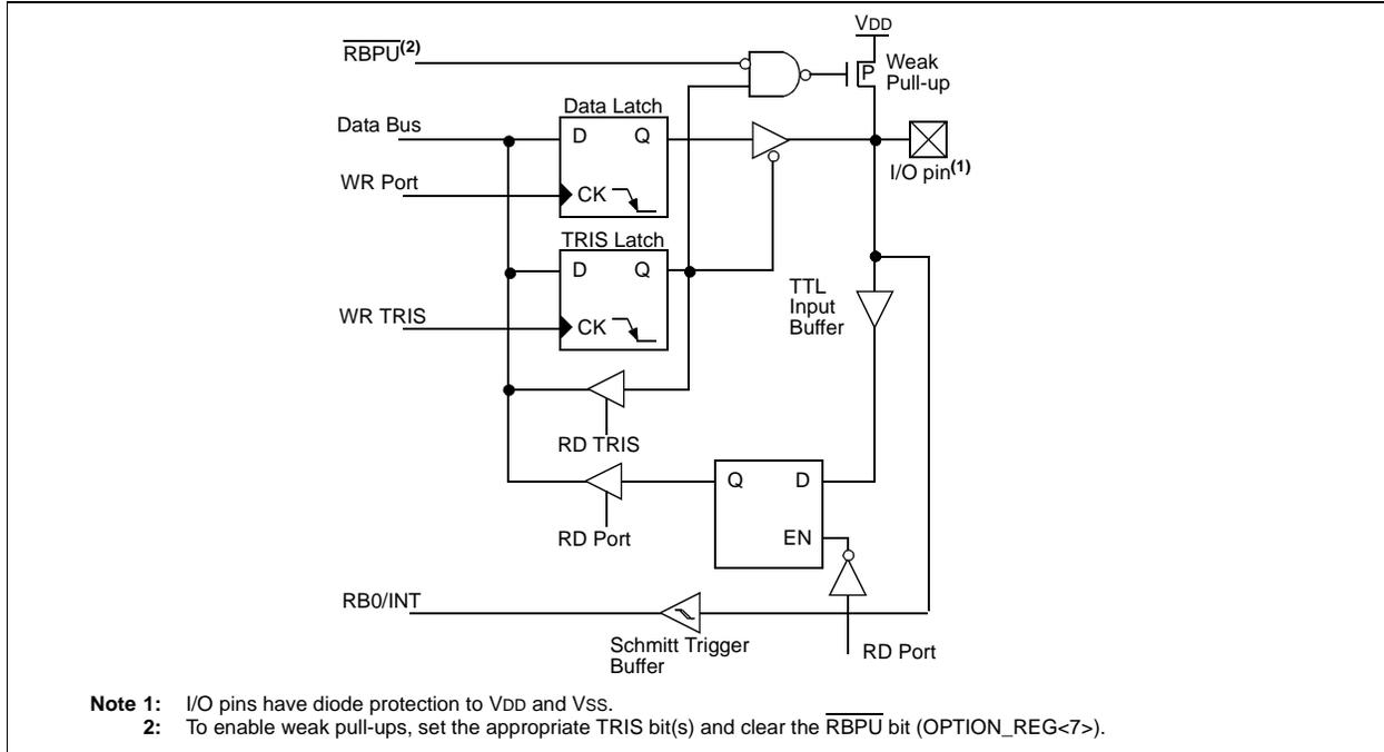
**FIGURE 9-6: BLOCK DIAGRAM OF RB3 PIN**
