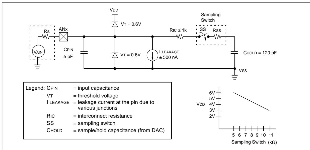
To calculate the minimum acquisition time, Equation 17-1 may be used. This equation assumes that 1/2 LSB error is used (1024 steps for the A/D). The 1/2 LSB error is the maximum error allowed for the A/D to meet its specified resolution.
