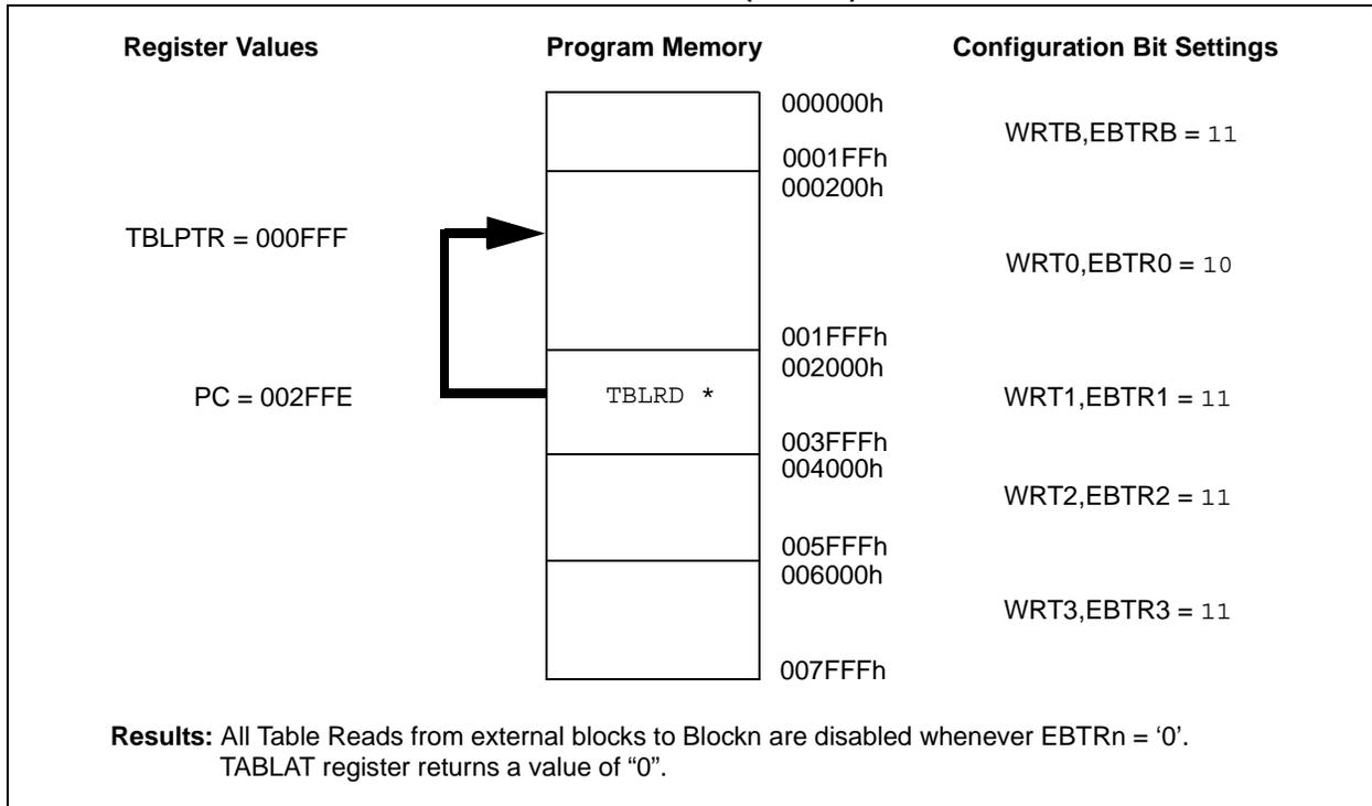
**FIGURE 19-6: EXTERNAL BLOCK TABLE READ (EBTRn) ALLOWED**
