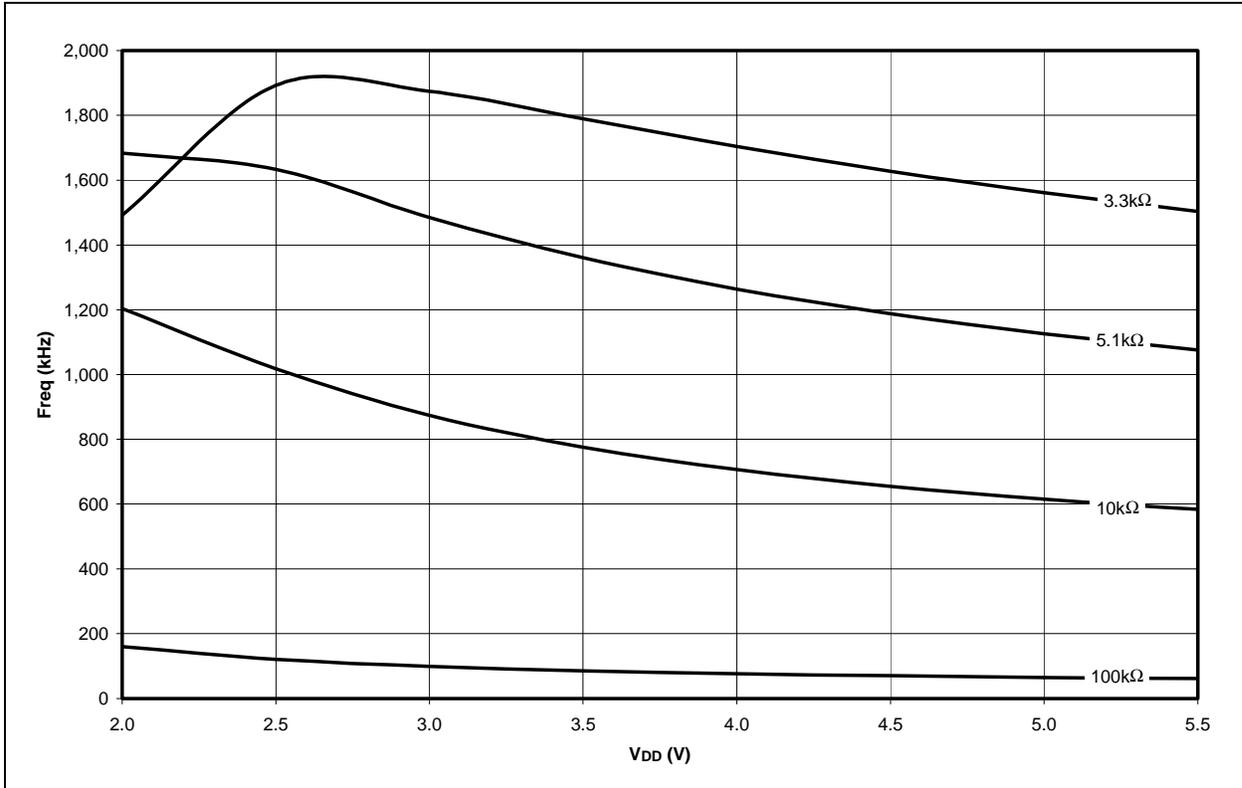
**FIGURE 23-14: AVERAGE  $F_{osc}$  vs.  $V_{DD}$  FOR VARIOUS VALUES OF R
