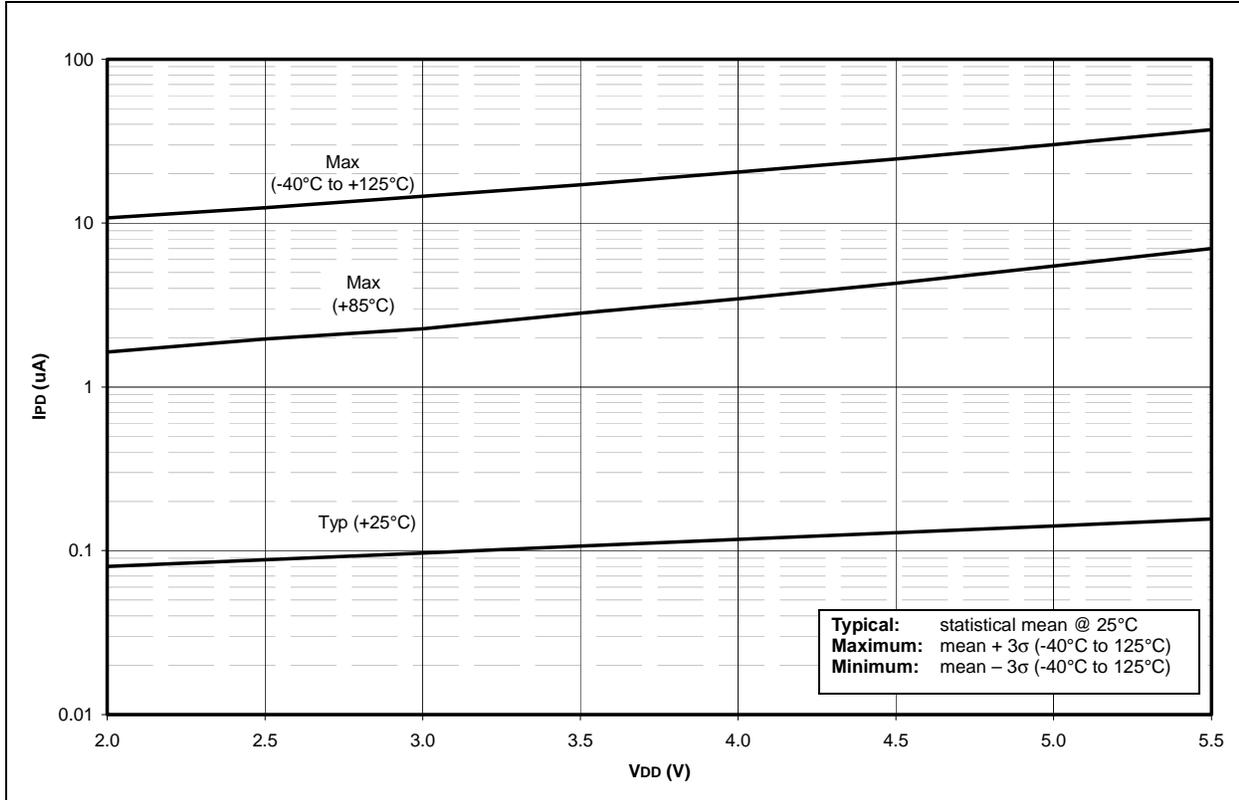
**FIGURE 23-16: ΔI<sub>BOR</sub> vs. V<sub>DD</sub> OVER TEMPERATURE (BOR ENABLED, V<sub>BOR</sub> = 2.00 - 2.16V)**
