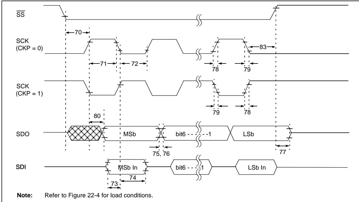
**TABLE 22-13: EXAMPLE SPI MODE REQUIREMENTS (SLAVE MODE TIMING (CKE = 0))**
