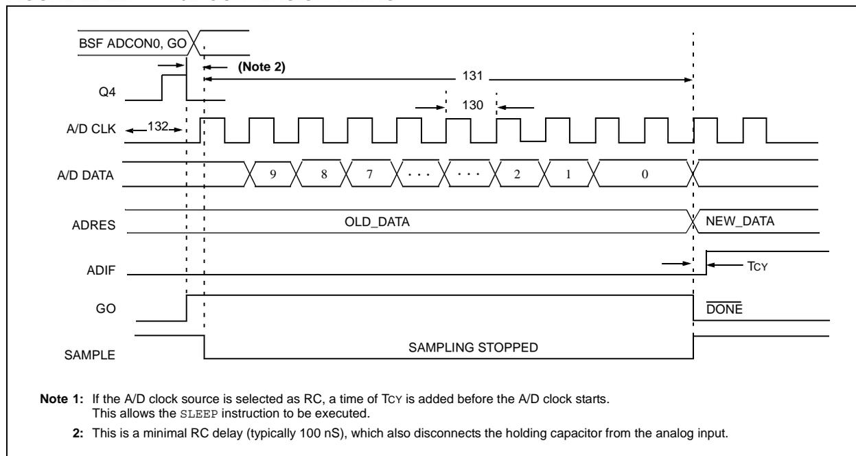
**Note 1:** If the A/D clock source is selected as RC, a time of  $T_{cy}$  is added before the A/D clock starts. This allows the SLEEP instruction to be executed.
