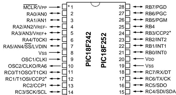
\* RB3 is the alternate pin for the CCP2 pin multiplexing.
