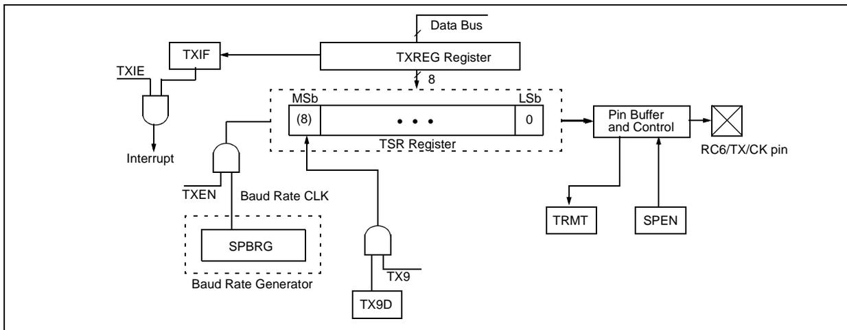
**FIGURE 16-2: ASYNCHRONOUS TRANSMISSION**
