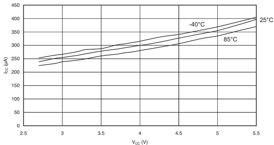
**Figure 184.** AREF External Reference Current vs.  $V_{CC}$
