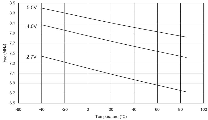
**Figure 171.** Calibrated 8MHz RC Oscillator Frequency vs.  $V_{CC}$
