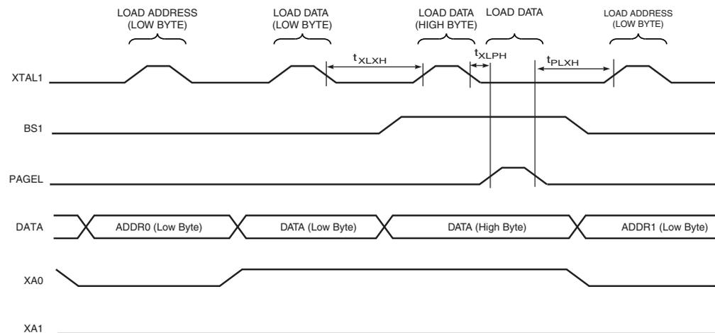
Note: 1. The timing requirements shown in Figure 109 (that is,  $t_{DVXH}$ ,  $t_{XHXL}$ , and  $t_{XLDX}$ ) also apply to loading operation
