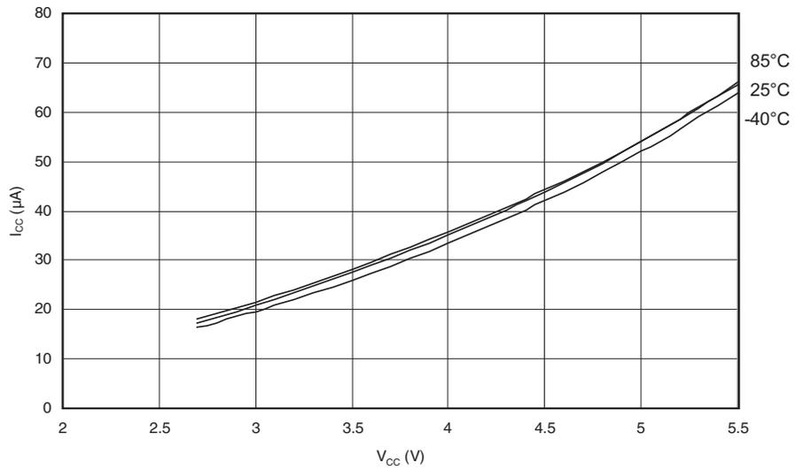
**Figure 187.** Analog Comparator Current vs.  $V_{CC}$
