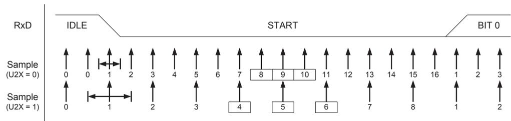
When the clock recovery logic detects a high (idle) to low (start) transition on the RxD line, the start bit detection sequence is initiated. Let sample 1 denote the first zero-sample as shown in
