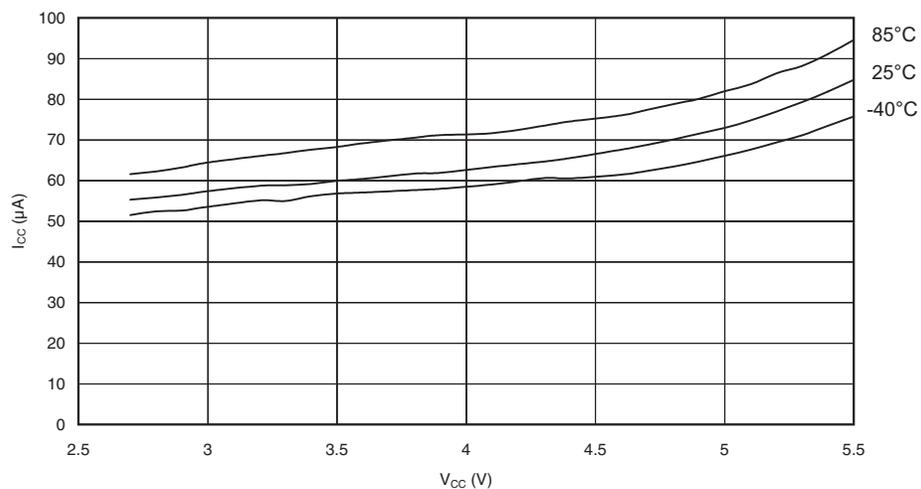
**Figure 188.** Programming Current vs.  $V_{CC}$
