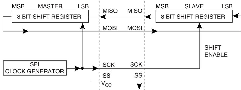
The system is single buffered in the transmit direction and double buffered in the receive direction. This means that bytes to be transmitted cannot be written to the SPI Data Register before the entire shift cycle is completed. When receiving data, however, a received character must be read from the SPI Data Register before the next character has been completely shifted in. Otherwise, the first byte is lost.
