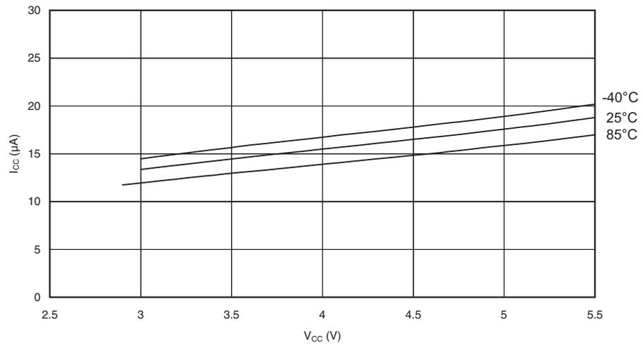
**Figure 183.** ADC Current vs.  $V_{CC}$  ( $A_{REF} = AV_{CC}$ )
