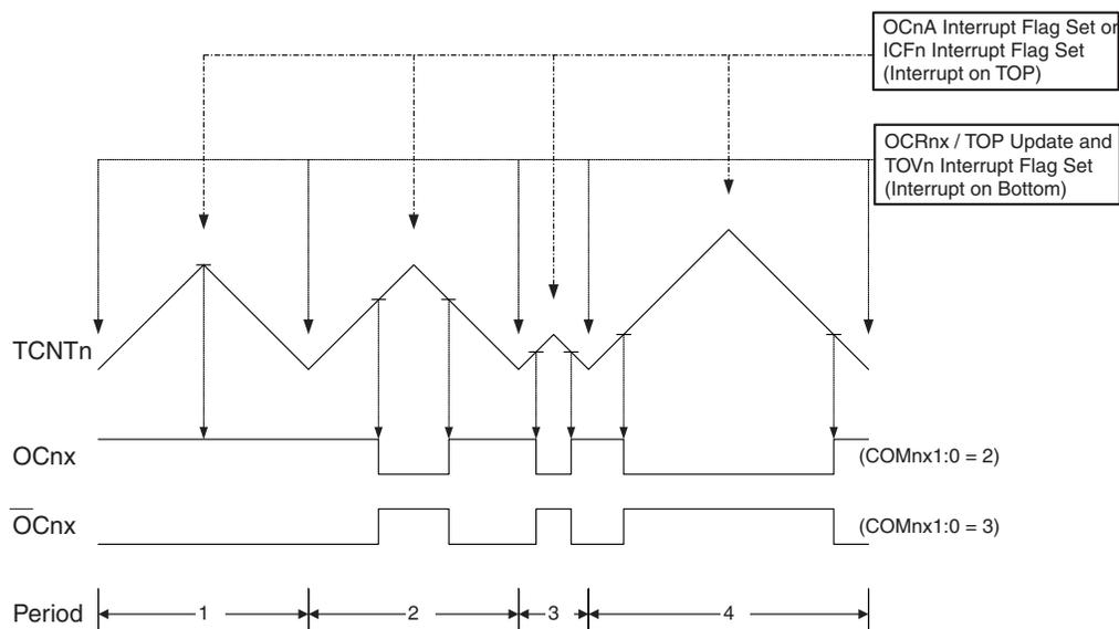
The Timer/Counter Overflow Flag (TOV1) is set at the same timer clock cycle as the OCR1x Registers are updated with the double buffer value (at BOTTOM). When either OCR1A or ICR1 is used for defining the TOP value, the OC1A or ICF1 Flag set when TCNT1 has reached TOP. The Interrupt Flags can then be used to generate an interrupt each time the counter reaches the TOP or BOTTOM value.
