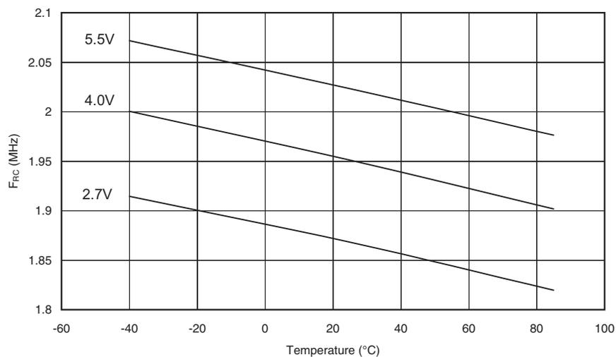
**Figure 177.** Calibrated 2MHz RC Oscillator Frequency vs.  $V_{CC}$
