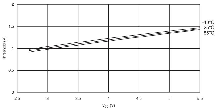
**Figure 157.** I/O Pin Input Hysteresis vs.  $V_{CC}$
