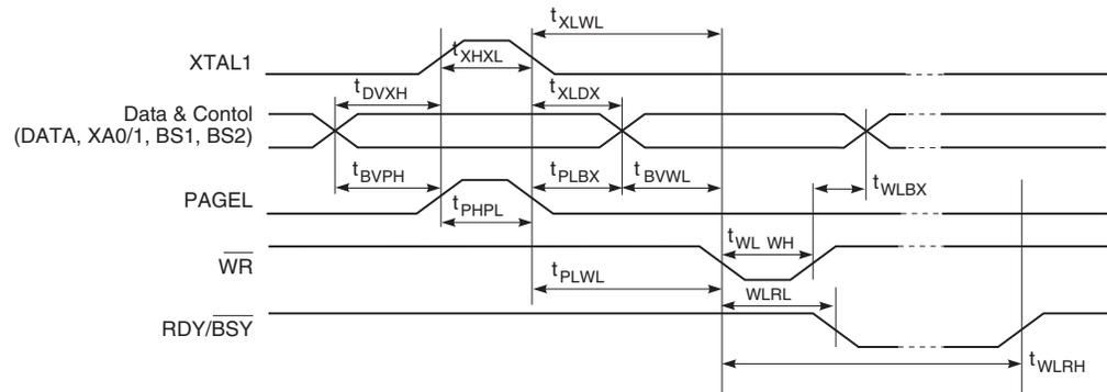
**Figure 110.** Parallel Programming Timing, Loading Sequence with Timing Requirements<sup>(1)</sup>
