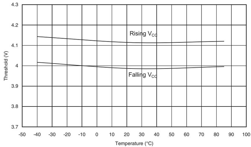
**Figure 165. BOD Thresholds vs. Temperature (BOD Level is 2.7V)**
