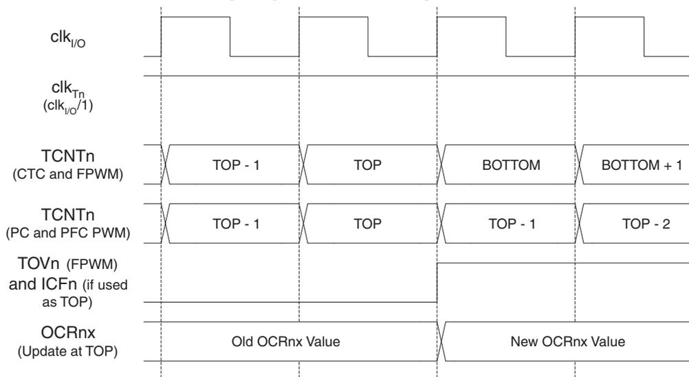
Figure 44 shows the same timing data, but with the prescaler enabled.
