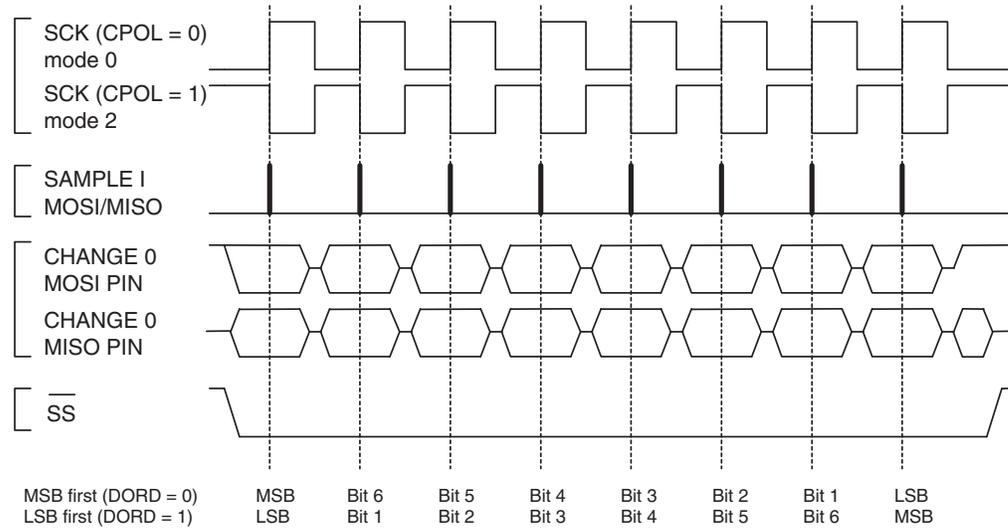
**Figure 60. SPI Transfer Format with CPHA = 1**
