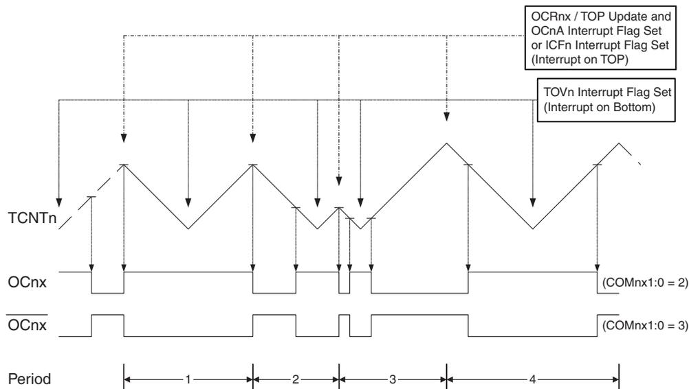
The Timer/Counter Overflow Flag (TOV1) is set each time the counter reaches BOTTOM. When either OCR1A or ICR1 is used for defining the TOP value, the OC1A or ICF1 Flag is set accordingly at the same timer clock cycle as the OCR1x Registers are updated with the double buffer value (at TOP). The Interrupt Flags can be used to generate an interrupt each time the counter reaches the TOP or BOTTOM value.
