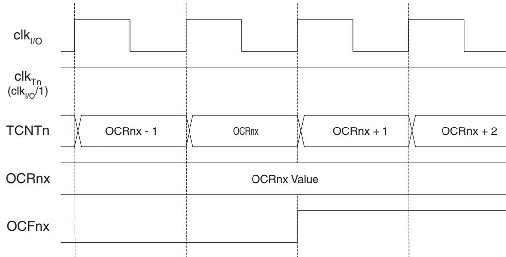
[Figure 42](#) shows the same timing data, but with the prescaler enabled.
