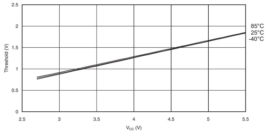
**Figure 163.** Reset Input Pin Hysteresis vs.  $V_{CC}$
