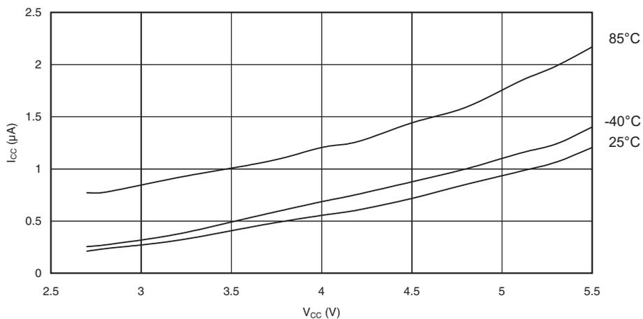
**Figure 133.** Power-down Supply Current vs.  $V_{CC}$  (Watchdog Timer Enabled)
