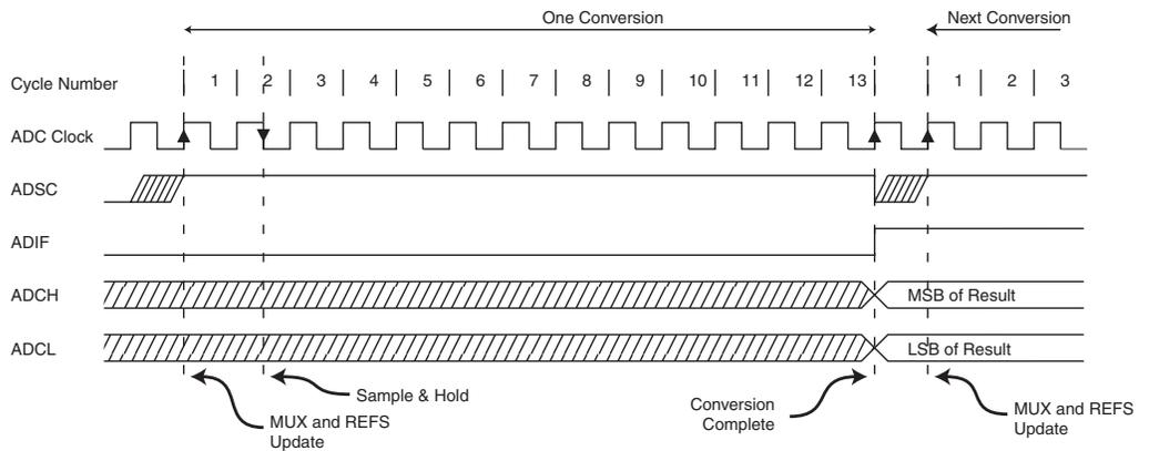
**Figure 94.** ADC Timing Diagram, Free Running Conversion
