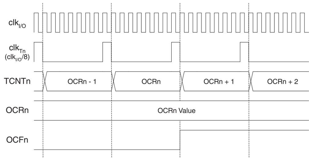
Figure 55 shows the setting of OCF2 and the clearing of TCNT2 in CTC mode.
