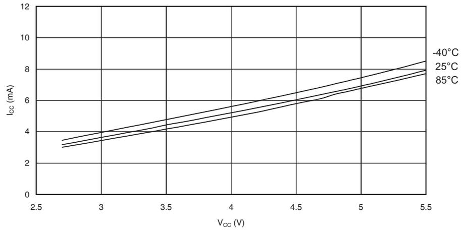
**Figure 122.** Active Supply Current vs.  $V_{CC}$  (Internal RC Oscillator, 2MHz)
