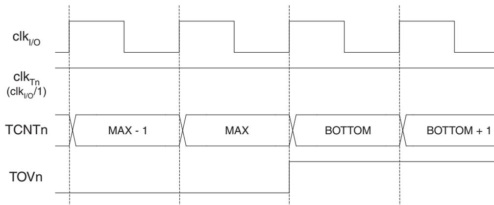
Figure 53 shows the same timing data, but with the prescaler enabled.
