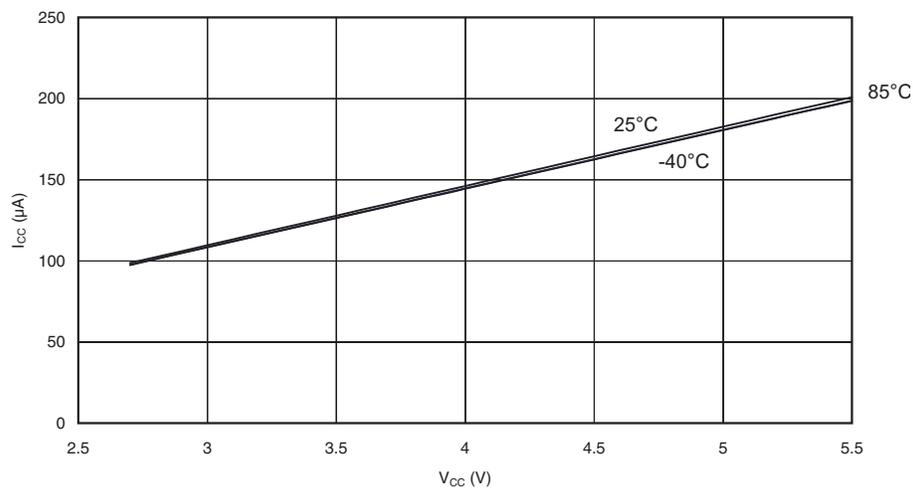
**Figure 185.** 32kHz TOSC Current vs.  $V_{CC}$  (Watchdog Timer Disabled)
