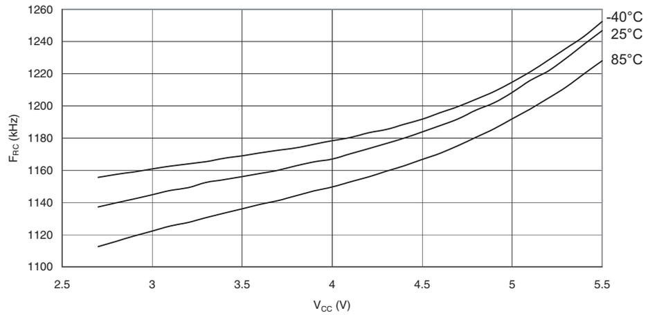
**Figure 170.** Calibrated 8MHz RC Oscillator Frequency vs. Temperature
