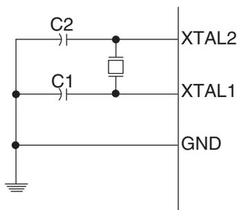
The Oscillator can operate in three different modes, each optimized for a specific frequency range. The operating mode is selected by the fuses CKSEL3..1 as shown in [Table 4](#).
