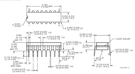
16-Lead Ceramic Dual-in-Line (J) Order Number LM1575J-3.3/883, LM1575J-5.0/883, LM1575J-12/883, LM1575J-15/883, or LM1575J-ADJ/883 **NS Package Number J16A**
