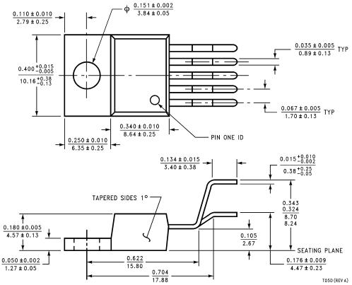
Bent, Staggered 5-Lead TO-220 (T)
