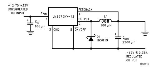
FIGURE 10. Inverting Buck-Boost Develops -12V
