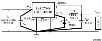
$C_{\text{IN}}$  — 100  $\mu\text{F},\,75\text{V},\,\text{Aluminum Electrolytic}$
