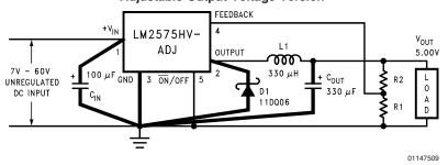
$$V_{OUT} = V_{REF} \left( 1 + \frac{R2}{R1} \right)$$
